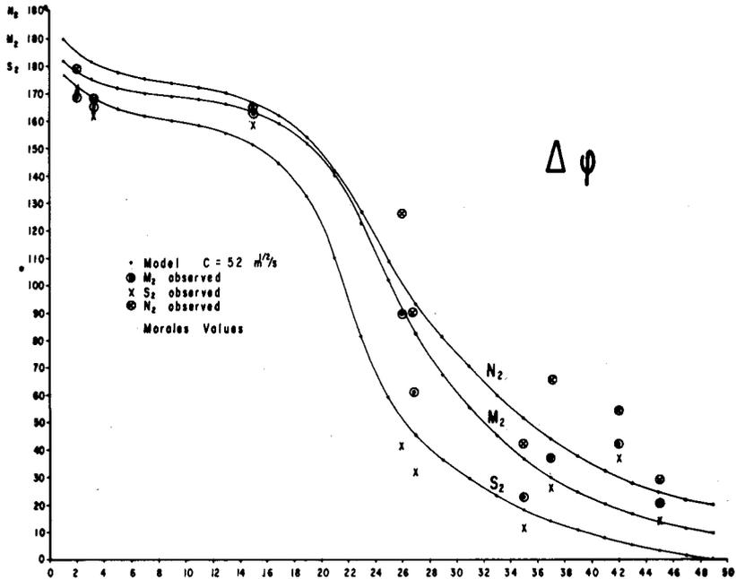
Fig. 7. Comparison between the phase differences predicted by the model and the constants reviewed by Morales for  $N_2$ ,  $M_2$ , and  $S_2$ .
