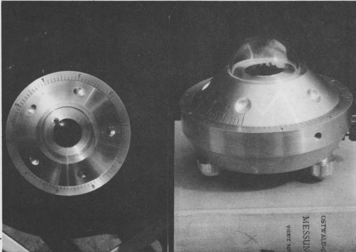
Fig. 2. Photograph of a pyranometer with sensitivity and time constant capable of being continuously varied.
