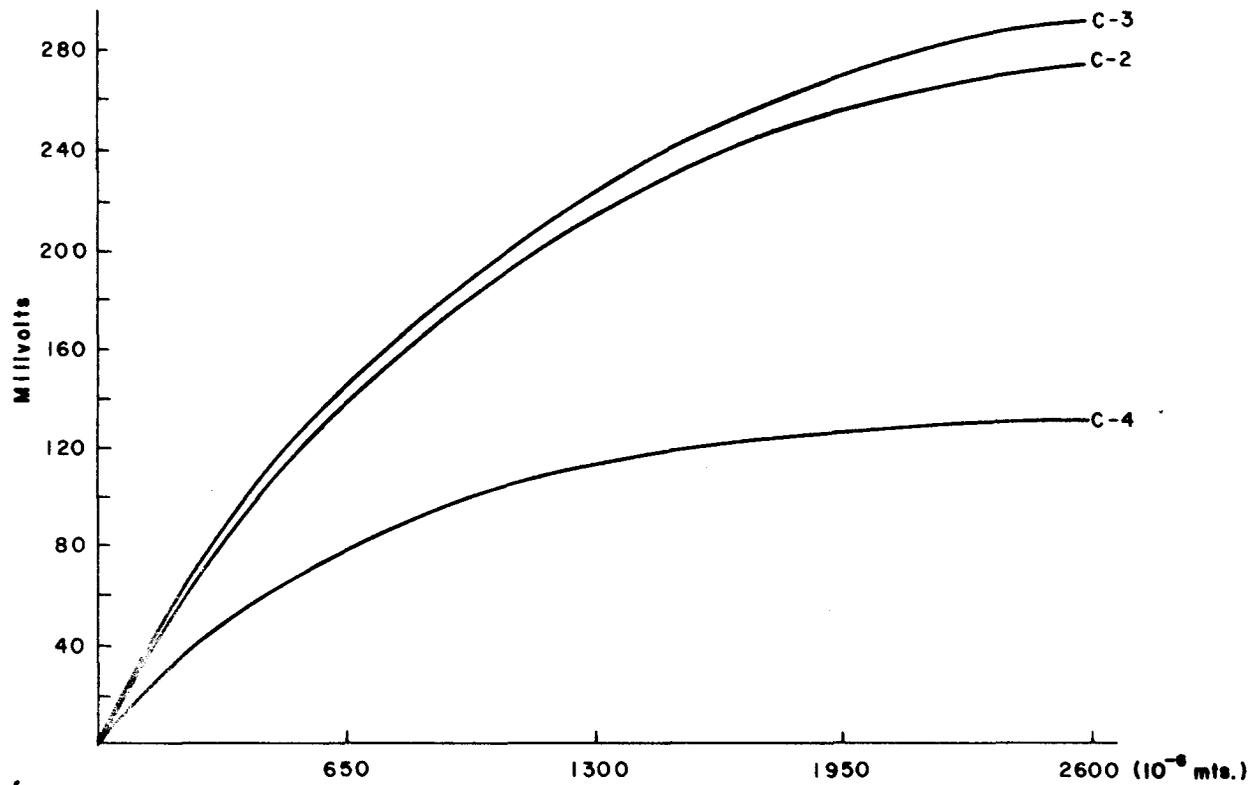
Fig. 4. Sensitivity vs. piston position from the top under a constant level of radiation (1.917 Langley/min.).
