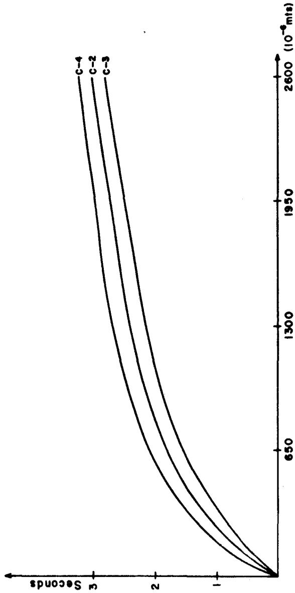
Fig. 5. Variation of time constant in terms of piston position from the top.
