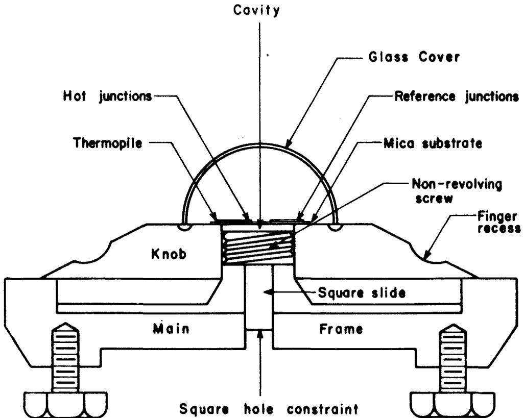
Fig. 3. Diagram of the pyranometer.
