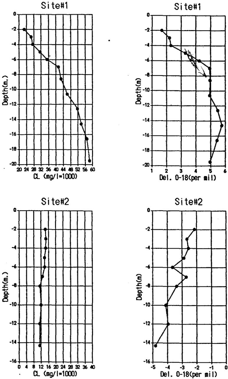
Fig. 14. Vertical profiles of Cl and <sup>18</sup>O.
