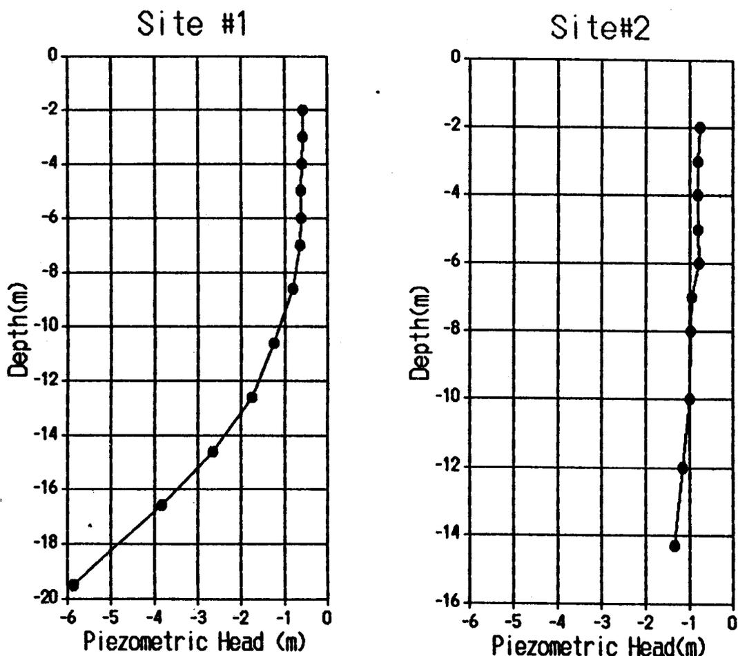
Fig. 13. Piezometric head profiles at Sites 1 and 2.
