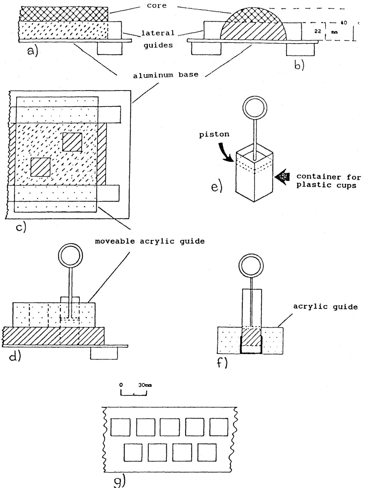
Fig. 3. Paleomagnetic sampling equipment. Schematic view of major parts used in sub-sampling: (a,b) base for half-cores (side view), (c,d) moveable guide for piston, (d,e,f) piston system for sampling, (g) sample separation (15 mm). Non-magnetic plastic cubes are about 10 cc.
