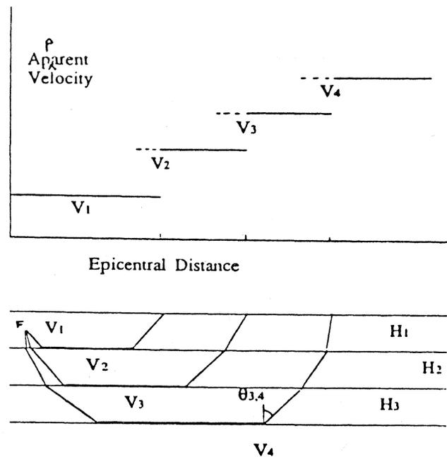
Fig. 2. Relationship between a hypothetical crustal model and its resulting minimum apparent velocity plot. Raypaths produced by a source point F are critically refracted at layers of thickness  $H_i$  with seismic velocities  $V_i$ . These critically refracted waves are recorded at different epicentral distances with a corresponding minimum apparent velocity.
