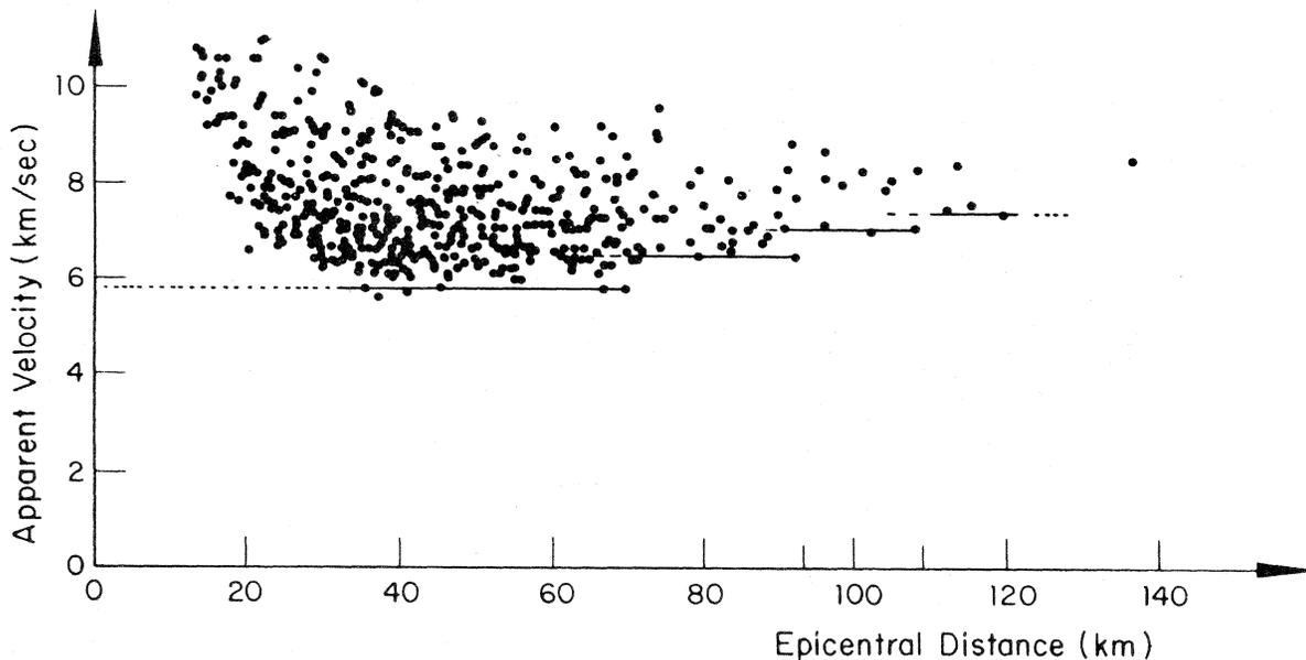
Fig.3. Resulting minimum apparent velocity plot. Dots represent observed apparent velocity arrivals as a function of epicentral distance. Four distinct layers are identified (solid lines). The dashed lines represent epicentral distances where no sampling of arrival times was available.
