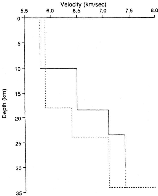
Fig. 4. Seismic velocity structure of the coast of Guerrero as a function of depth resulting from this study (solid line) compared with the results of Valdés *et al.* (1982) (dashed line). The dotted line in the resulting velocity profile indicates depths for which no sampling of refracted waves was available (see Figure 3).
