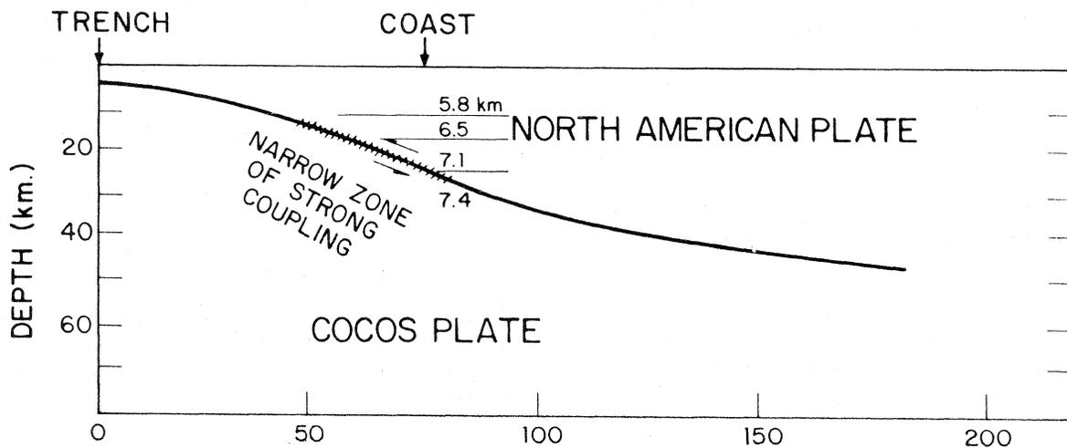
Fig. 5. Geometry of the subducted slab beneath the coast of central Guerrero. The depth and velocity of the layers obtained in the study are shown in the figure. Notice that near the coastline the depth of the deepest layer sampled corresponds approximately to the interplate contact (hatched line), suggesting the forearc of the overriding plate is devoid of mantle and the lower crust of the North American plate rests directly on the Cocos plate.
