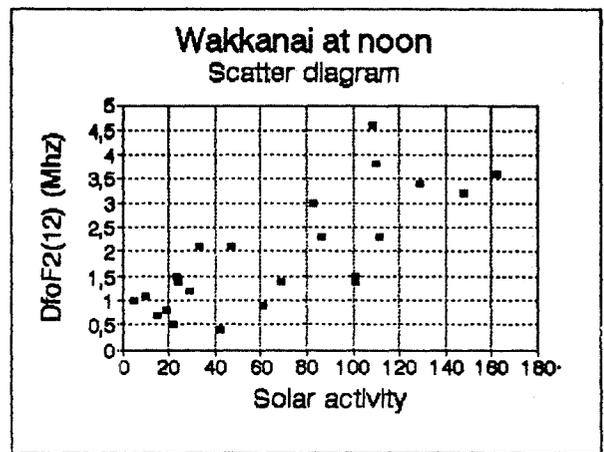
Fig. 3. Scatter diagrams for foF2(00) and foF2(12) versus solar activity for Dourbes (25 data years, above) and Wakkanai (23 data years, below). Both stations are in the northern hemisphere and have similar latitudes. The nocturnal adjustment is better than the diurnal. Wakkanai, at noon, shows the largest dispersion.
