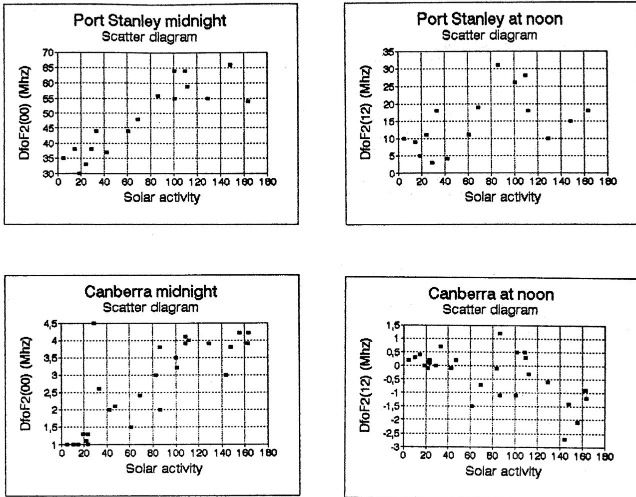
Fig. 4. Scatter diagrams for foF2(00) and foF2(12) versus solar activity for Canberra (27 data years, above) and Port Stanley (17 data years, below). Both stations are in the southern hemisphere and have similar latitudes. The nocturnal adjustment is better than the diurnal. Port Stanley, at noon, shows the largest dispersion.
