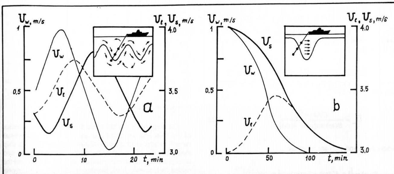
Fig. 3. Ship velocity changes ( $U_s$ ), according to log ( $U_l$ ) in the field of orbital currents ( $U_w$ ) of the internal sinusoidal waves (a) and (b) when the ship track is normal to the internal soliton front.
