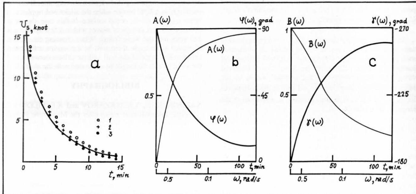
Fig. 2. (a) Experimental curve of slow-down of R.V. "Acad. N. Andreyev". The approximation of the same curve by formula (4) for  $\tau = 3.5$  min (5),  $\tau = 4$  min (6) and  $\tau = 5$  min (7), shown by symbols. (b) Amplitude-phase frequency slowing-down response of ship's  $A(\omega)$ ,  $\phi(\omega)$  and (c) log readings  $B(\omega)$ ,  $\gamma(\omega)$ , from the period of horizontal orbital currents.
