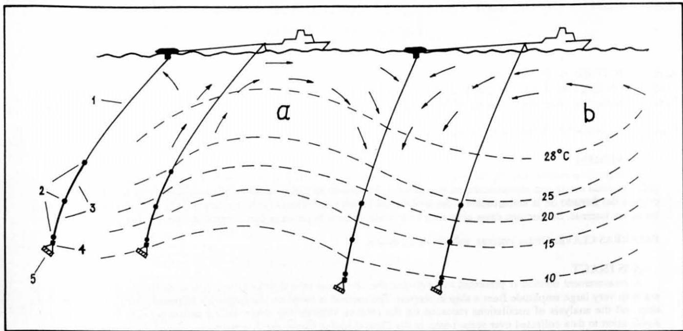
Fig. 1. Schema of the position of the towing systems TSMs on the thermocline, at the moment in which the ship is located on the field of orbital currents (a) with the same direction and (b) against the front of the internal waves of large amplitude. In the left part of the figure is shown a diagram of a towed system TSM: 1-cable, 2-thermistors, 3-sensors of temperature distribution, 4-pressure sensor, 5-submersion weight.
