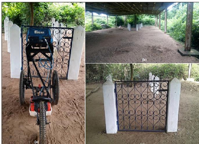
**Figure 4.** Photographs of the (a) GSSI (SIR-3000) GPR equipment with a 400 MHz antenna, (b) the entire burial site and the (c) Tomb area cordoned by the fence.
