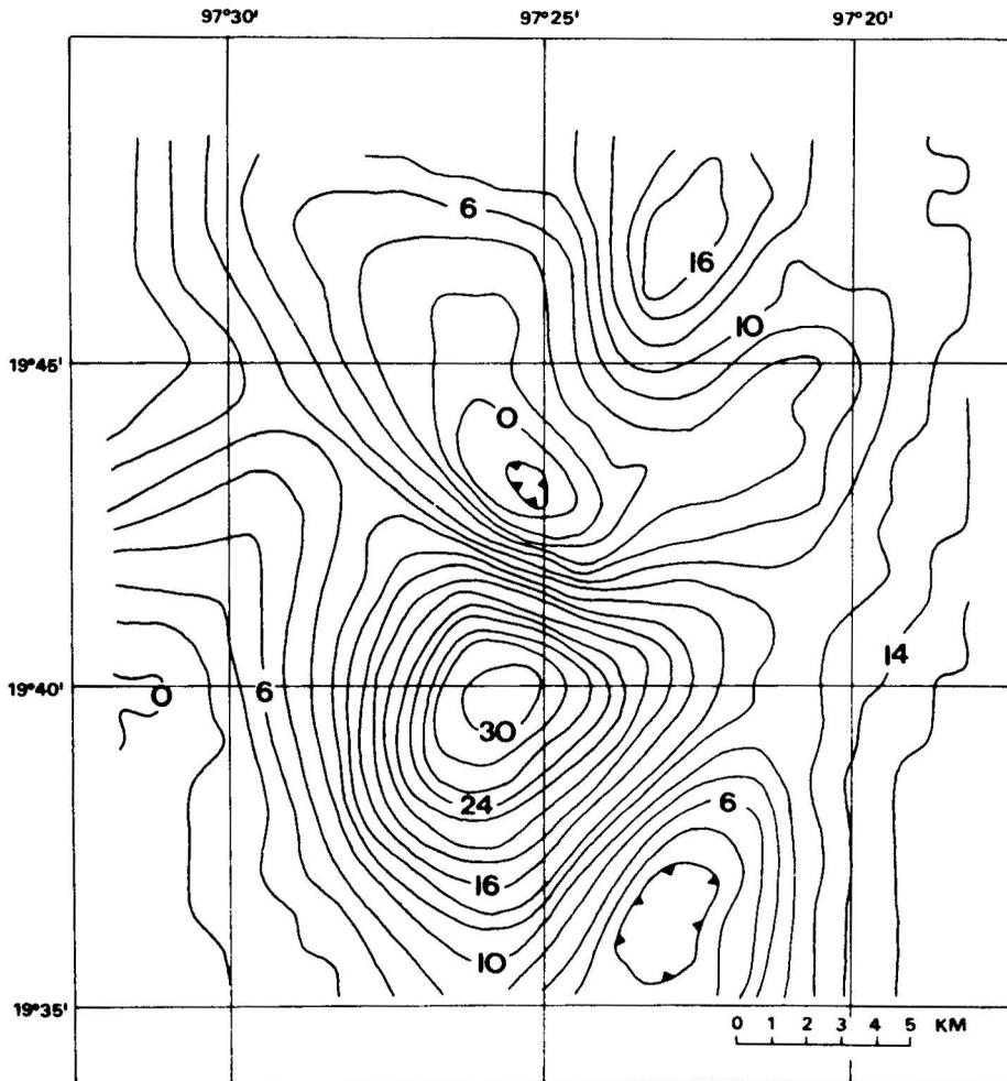
Figure 2. Upward continuation of the observed residual total field to a height of 2 km above ground level. Contour interval is 2 gammas.
