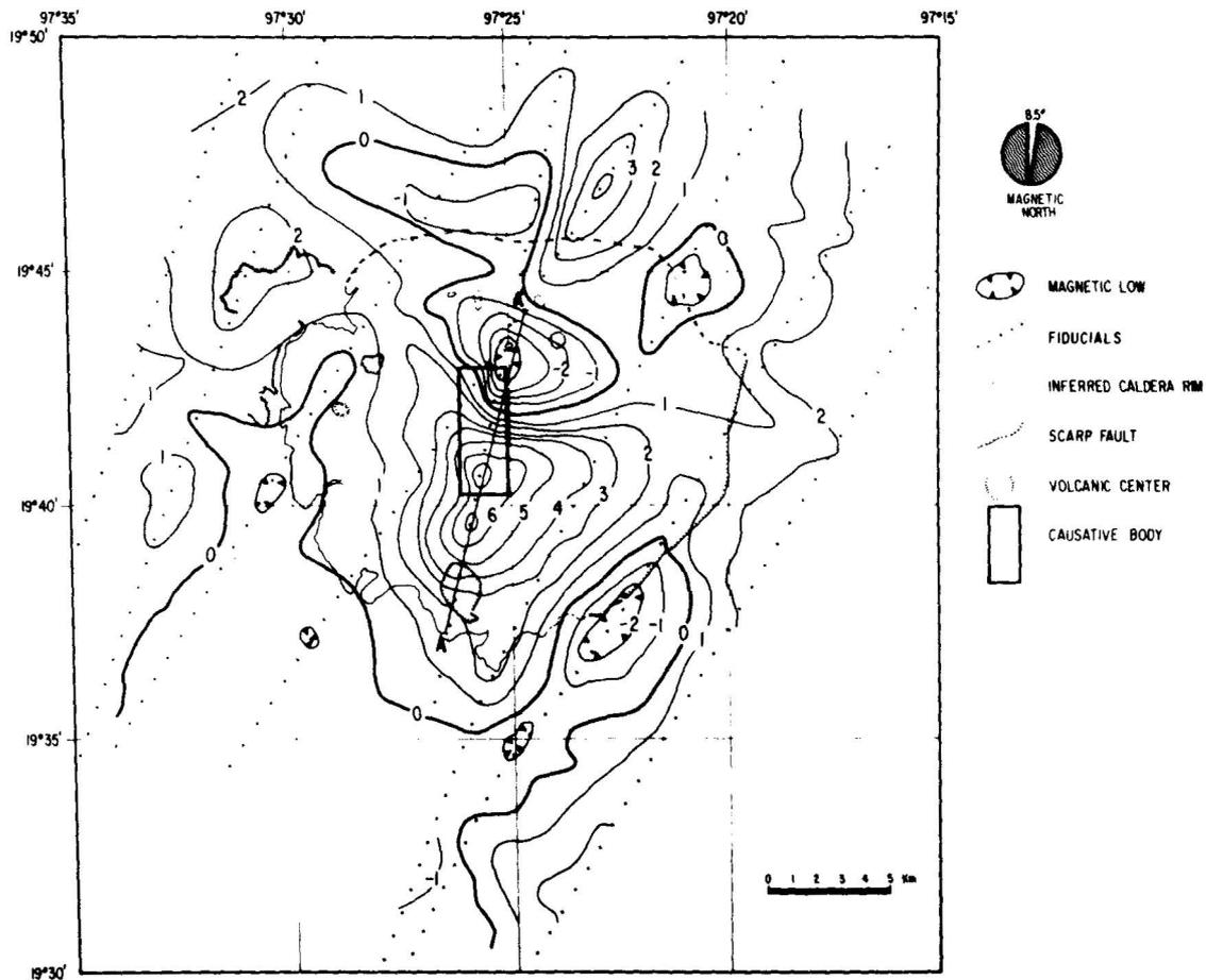
Figure 1. Three point average of total field, residual aeromagnetic map from Los Humeros caldera. Nominal flying altitude was 250 meters above terrain surface. Contour interval is 100 gammas. Flight lines, proposed causative body, major structural features and rim of the caldera (dashed where inferred) are shown.
