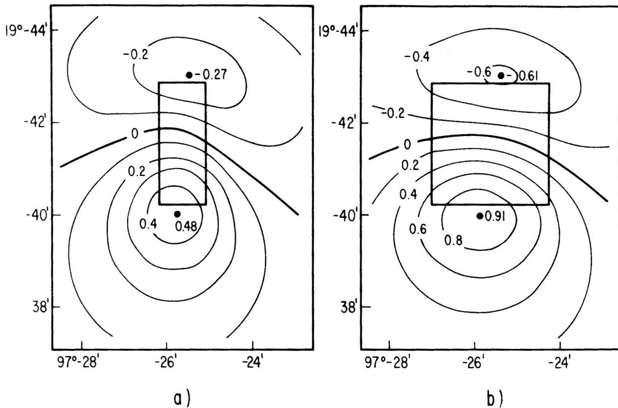
Figure 4. Normalized total magnetic intensity: a)  $\alpha = 5.0$  km,  $\beta = 2.0$  km; b)  $\alpha = 5.0$  km,  $\beta = 5.0$  km. All other parameters are the same as for Figure 3. Dots show maximum and minimum values of the normalized field.
