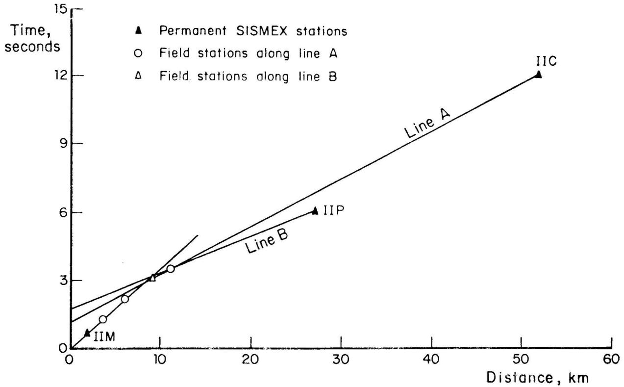
Fig. 2. Travel time - distance plot along lines A and B (Fig. 1).
