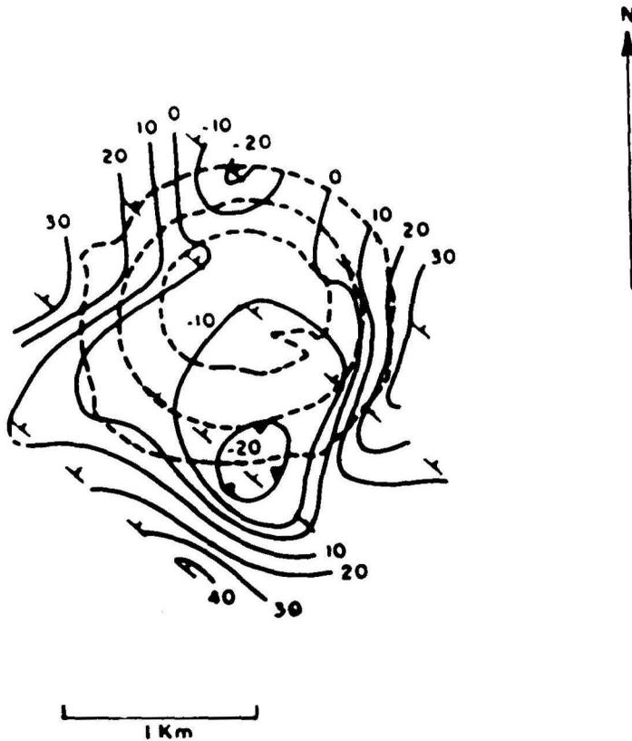
Fig. 5 (a). Total field intensity map for Tepexitl. Contour interval is 10 gammas. Total field values are obtained adding 43 660 gammas. Flight lines and points where readings were made are shown by fiducials. Concentric dashed lines delimit the rim of the structure.
