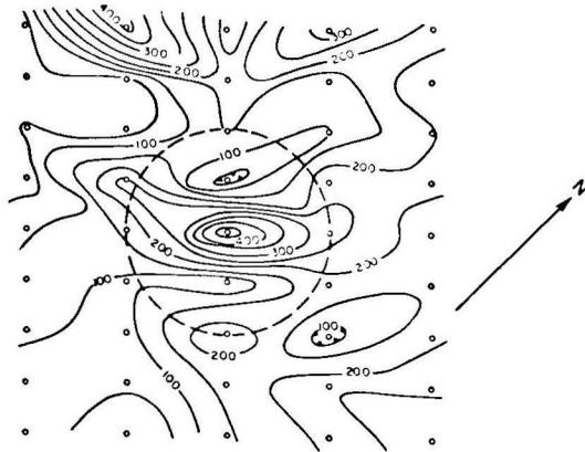
Fig. 5 (b). Vertical component map of the magnetic field (ground survey). Small circles denote reading stations; station interval is 300 m and line interval 600 m. Contour interval is 50 gammas.
