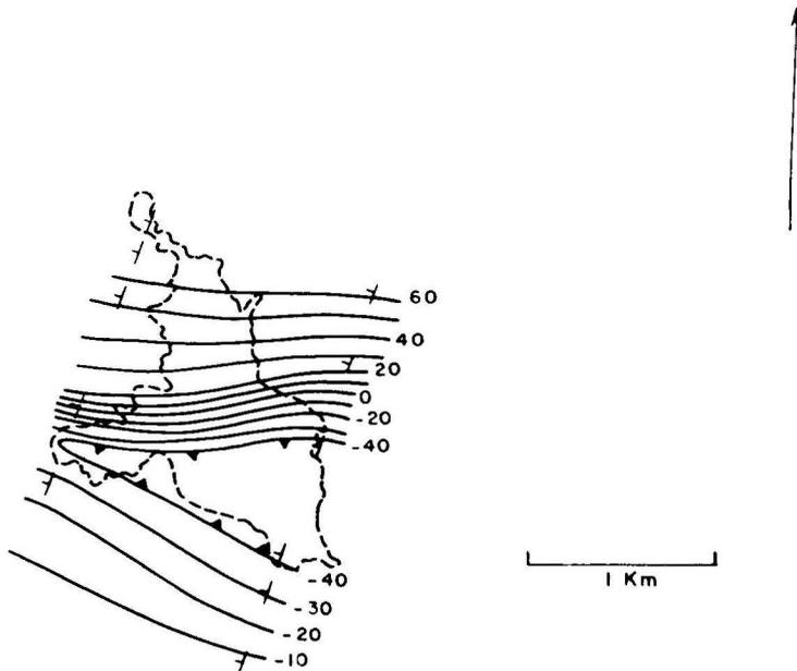
Fig. 6. Total field intensity map for La Campana. Total field values are obtained adding 43 560 gammas. Only two lines were flown; the response of this structure is a magnetic low.
