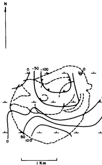
Fig. 9. Total intensity map for Volcán. Contour interval is 50 gammas. Total field values are obtained adding 43 560 gammas. The dashed lines within the structure denote surface features visible on Figure 7.
