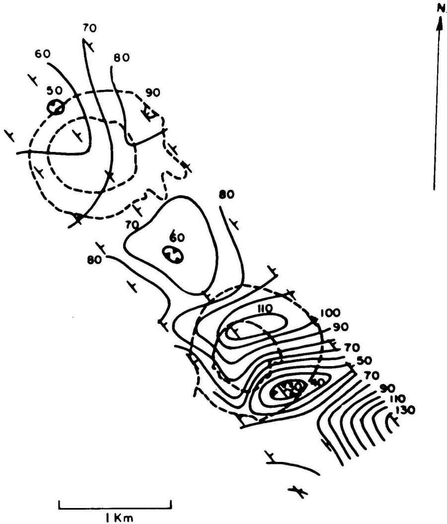
Fig. 13 (b). Total field intensity map for the Xalapazcos. Contour interval is 10 gammas. Total field values are obtained adding 43 360 gammas. Dashed lines represent top and bottom perimeters of these structures. A considerable difference in response is observed between the two Xalapazcos.
