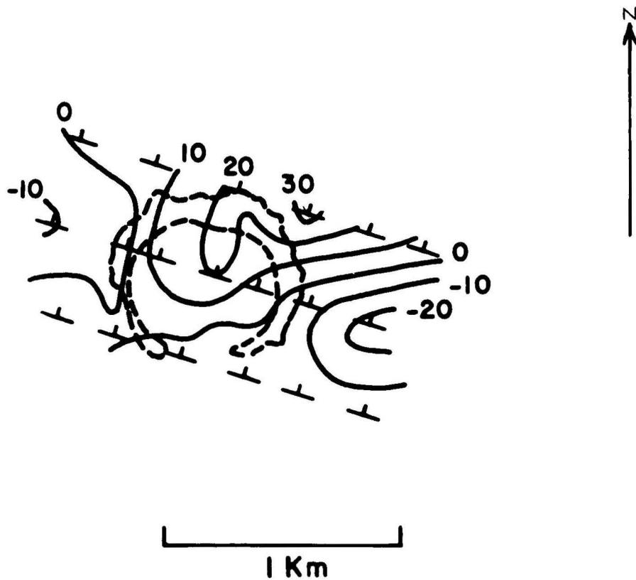
Fig. 8. Total field intensity map for Buenavista. Contour interval is 10 gammas. Total field values are obtained adding 43 560 gammas.
