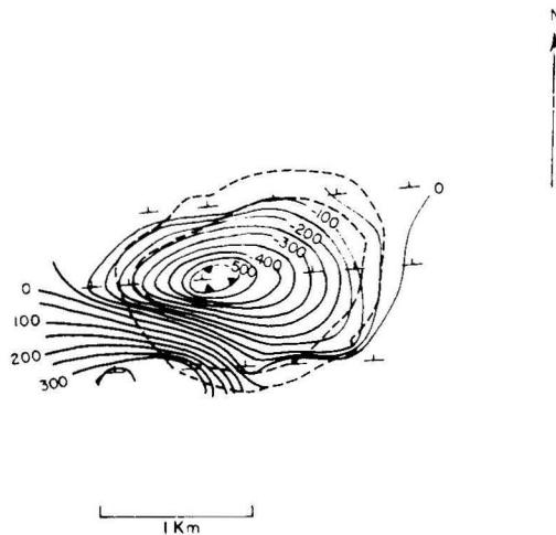
Fig. 11 (b). Total field intensity map for Tecuítlapa. Contour interval is 50 gammas. Total field values are obtained adding 43 360 gammas. Dashed lines delimit the rim of the structure.
