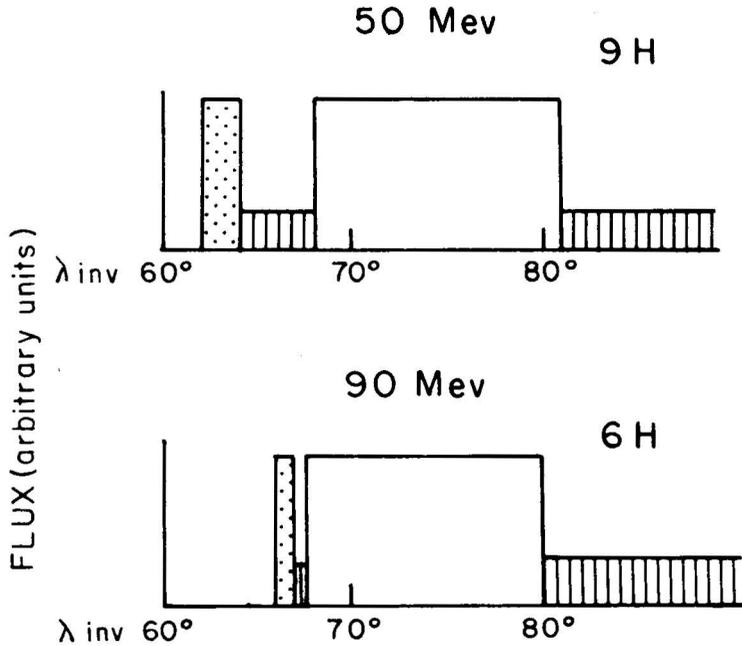
Figure 7. Theoretical monoenergetic flux profiles along two local time meridians. Illumination in absence of shielding by direct impact through front magnetopause is indicated by white areas; the pointed and striped latitudinal zones are illuminated respectively from dawn plasma sheet and by flux impinging under large pitch angles.
