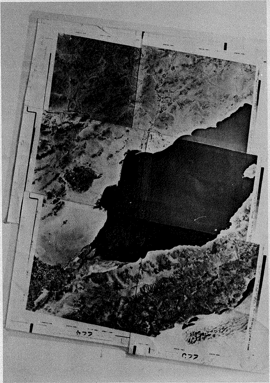
Fig. 1. Mosaic of electronically dodged 1:million scale prints of images in band 4 of September 28, 29, 30, 1972 showing the Sept. 30 plume at 10:45 am local time.
