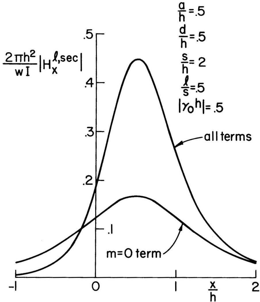
Figure 10. Normalized horizontal secondary magnetic field of a truncated cylinder for loop excitation.
