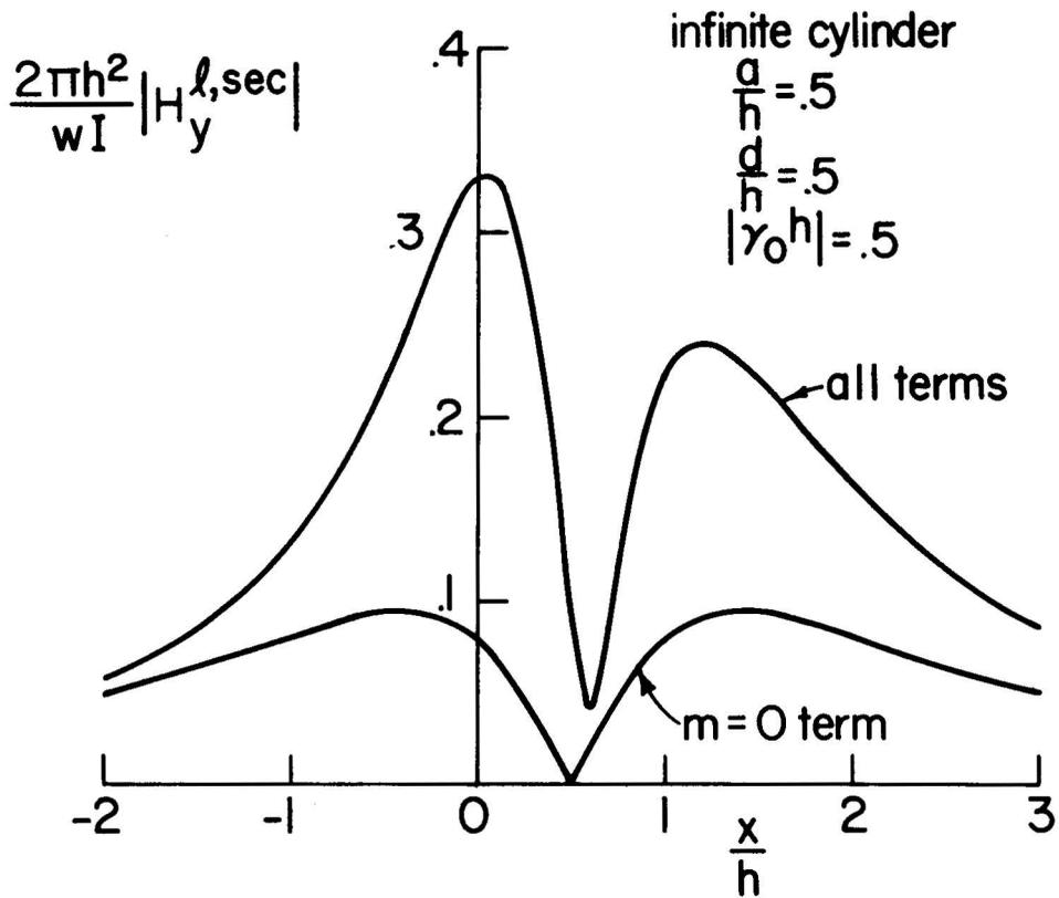
Figura 7. Normalized vertical secondary magnetic field of an infinite cylinder for loop excitation.
