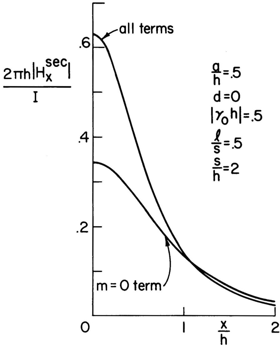
Figure 6. Normalized horizontal secondary magnetic field of a truncated cylinder for line source excitation.
