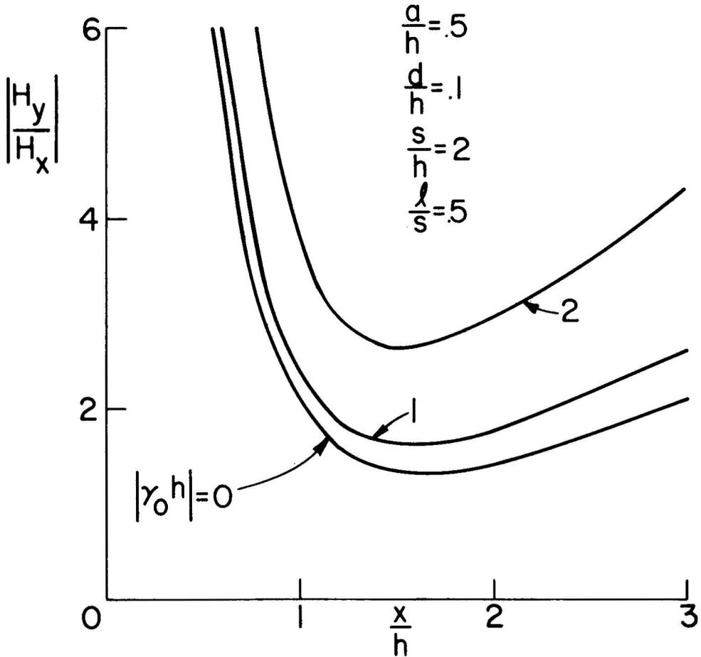
Figure 14. Effect of  $\gamma_0$  on the magnitude of the ratio of vertical to horizontal magnetic field (truncated cylinder case).
