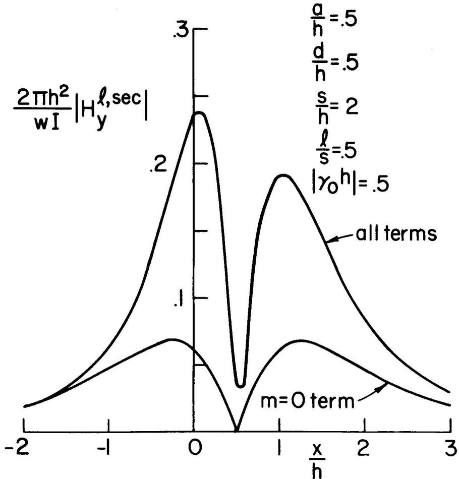
Figure 9. Normalized vertical secondary magnetic field of a truncated cylinder for loop excitation.
