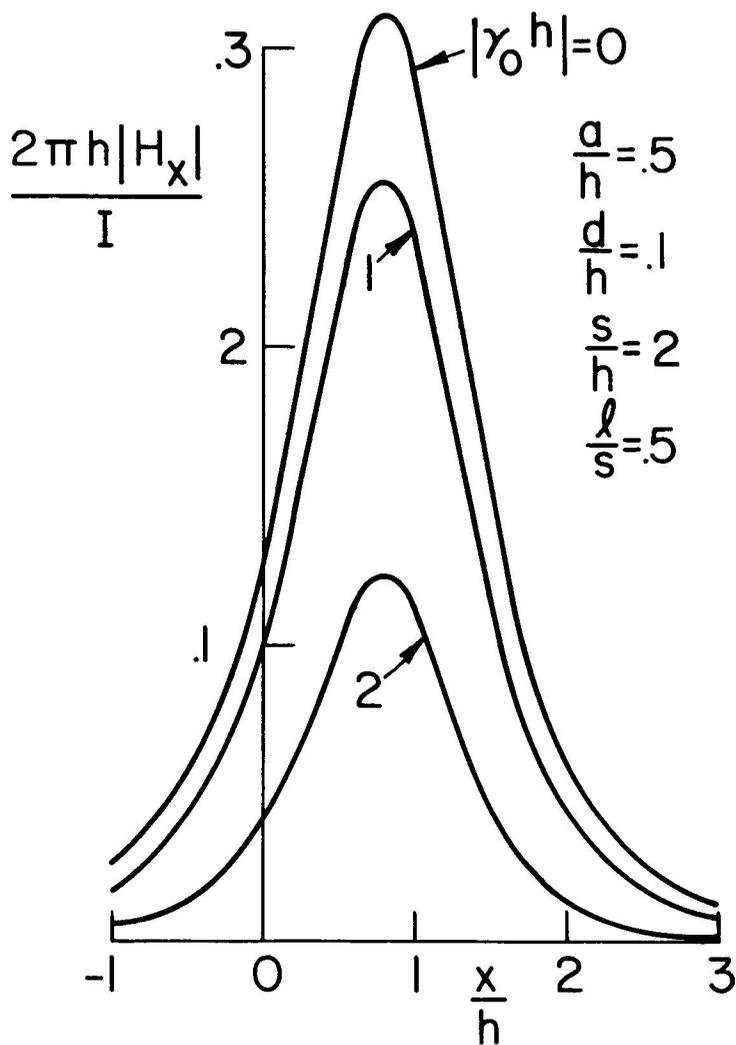
Figure 13. Effect of  $\gamma_0$  on the horizontal magnetic field for the truncated cylinder case.
