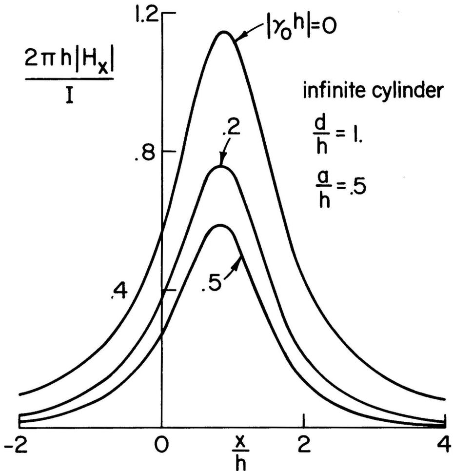
Figure 11. Effect of  $\gamma_0$  on the horizontal magnetic field for the infinite cylinder case.
