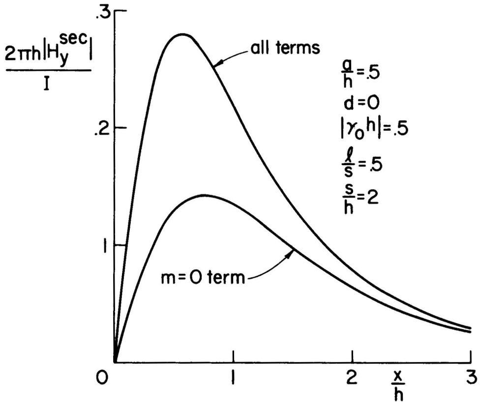
Figure 5. Normalized vertical secondary magnetic field of a truncated cylinder for line source excitation.
