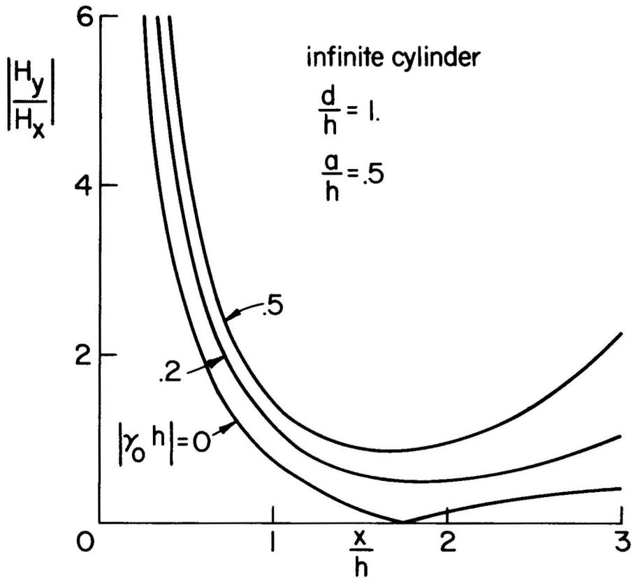
Figure 12. Effect of  $\gamma_0$  on the magnitude of the ratio of vertical to horizontal magnetic field (infinite cylinder case).
