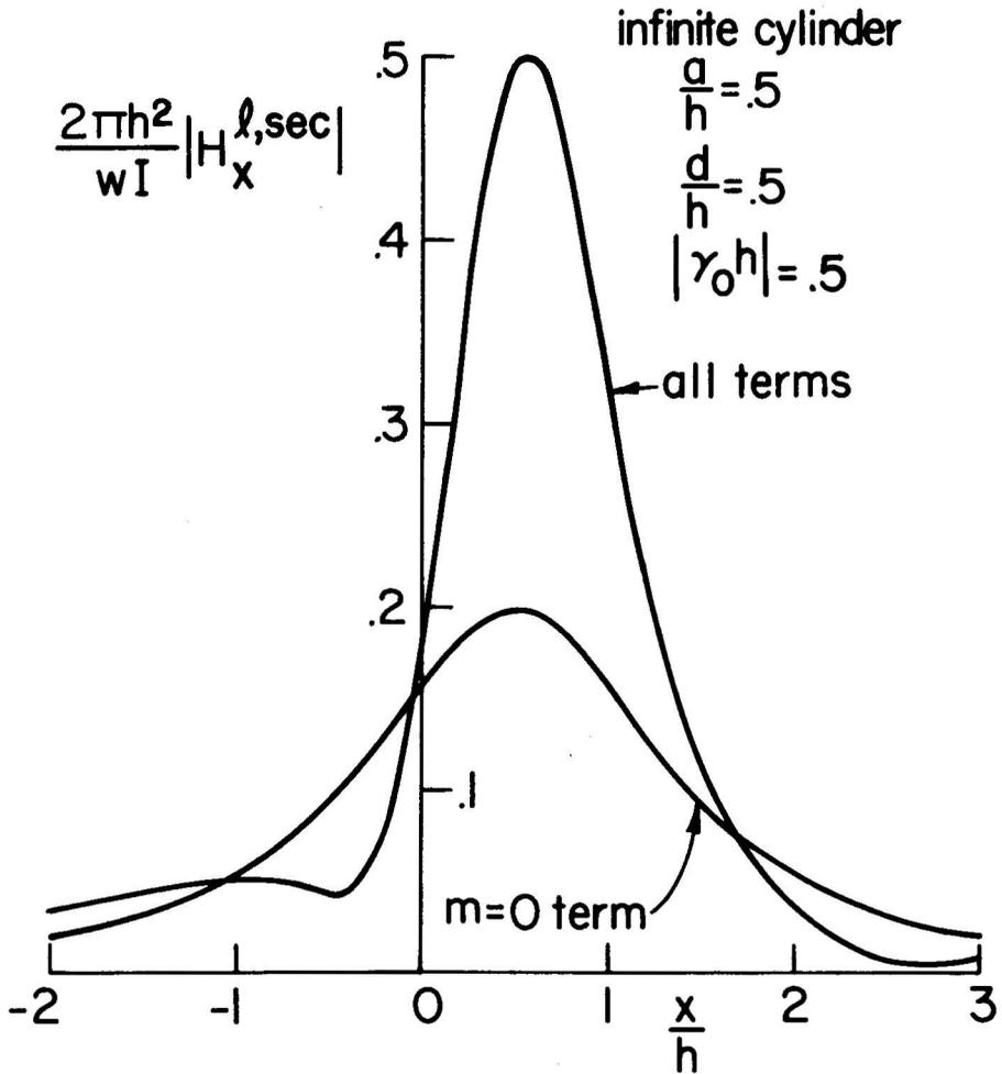
Figure 8. Normalized horizontal secondary magnetic field of an infinite cylinder for loop excitation.
