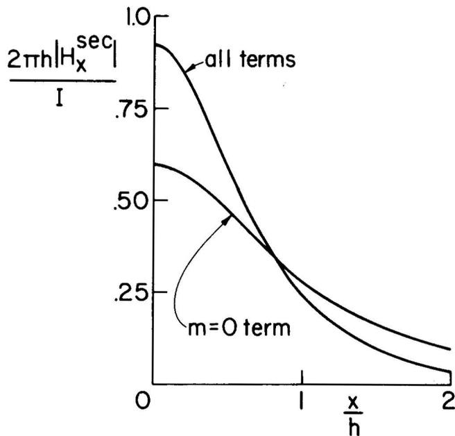
Figure 4. Normalized horizontal secondary magnetic field of an infinite cylinder for line source excitation.
