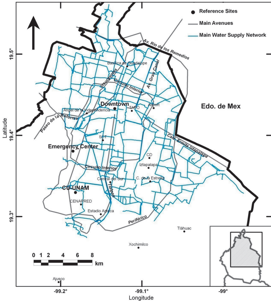
Figure 5. Distribution of Mexico City's water network.
