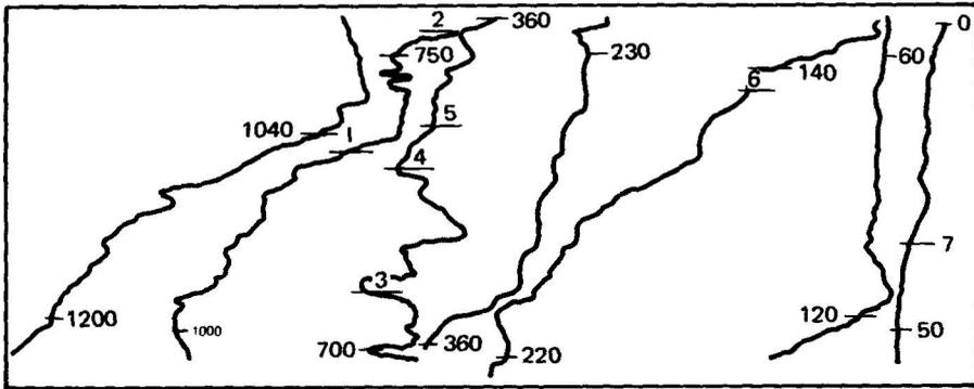
Figura 1. The conductivity profile in the upper 1 200 m layer of water in the tropical zone of the Indian Ocean during winter monsoon. Horizontal scale is the conductivity in arbitrary units (increases to the right). For convenience the profile is cut into 7 parts. Depths in metres are shown by figures.
