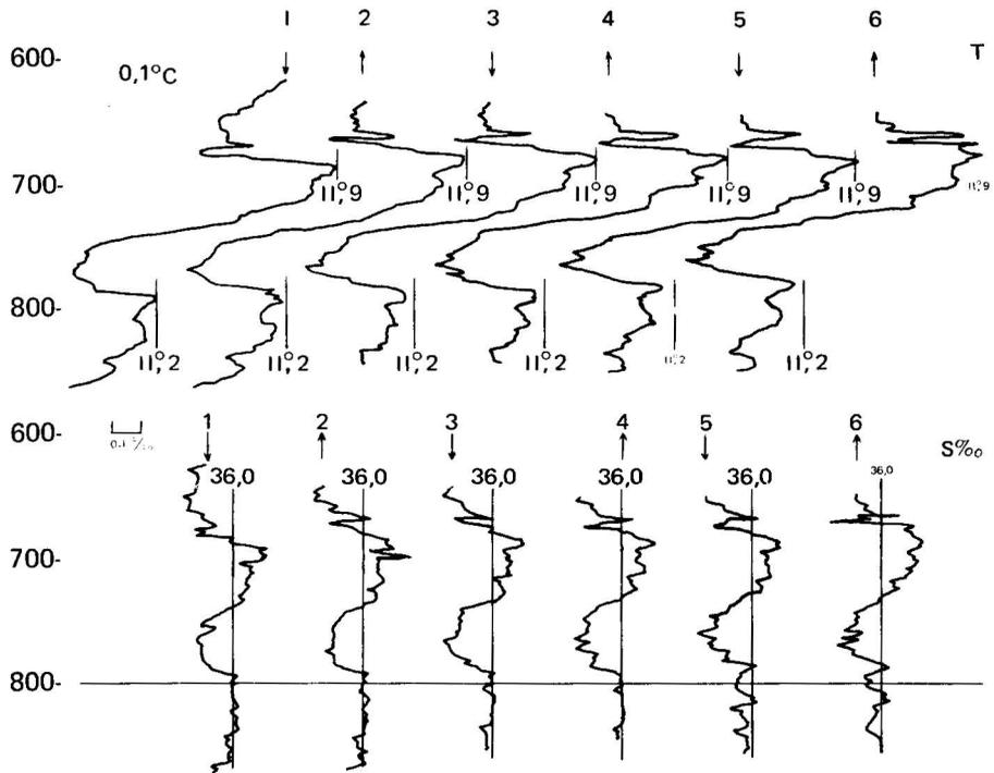
Figure 3. Six pairs of temperature and salinity profiles at depths of 650 to 850 m in Timor Sea measured with time lags of 30 min.
