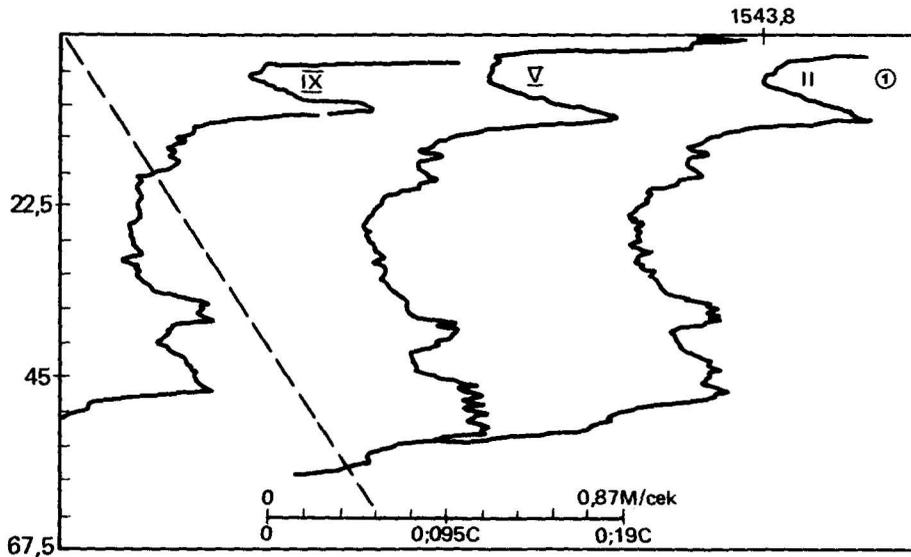
Figure 2. Three sound velocity profiles in the upper layer of the ocean measured with time lags of 10 min.
