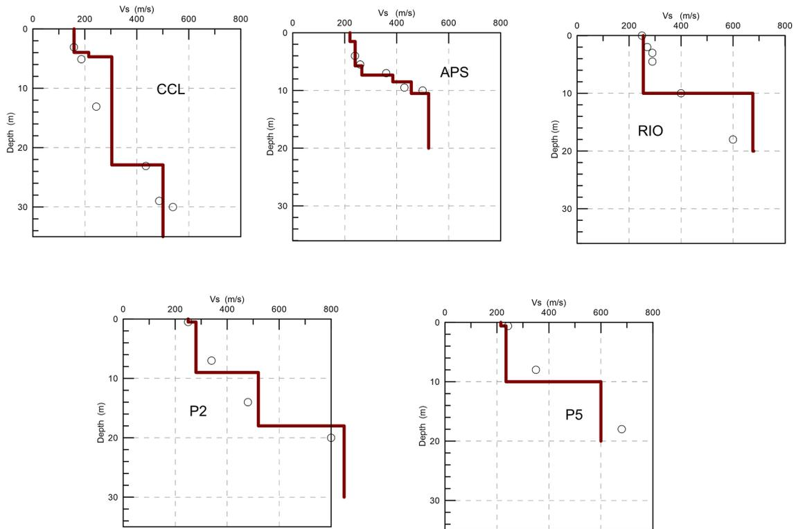
**Figure 9.** S-wave velocity profiles for five locations for which soil mechanics studies were available. The circles indicate the values obtained in those studies. The solid lines show the profile obtained from the inversion of the phase velocity dispersion curves observed at the corresponding location.
