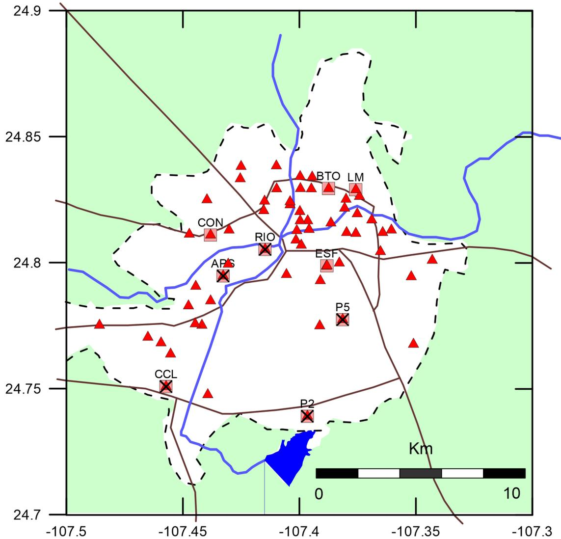
**Figure 3.** Location of HVSR measuring points (triangles). The white zone represents the urban sprawl of the city. Main streets and rivers are shown. Labeled squares indicate the sites where multi-channel measurements were made and velocity profiles were obtained. Crosses indicate places for which soil mechanics information is available.
