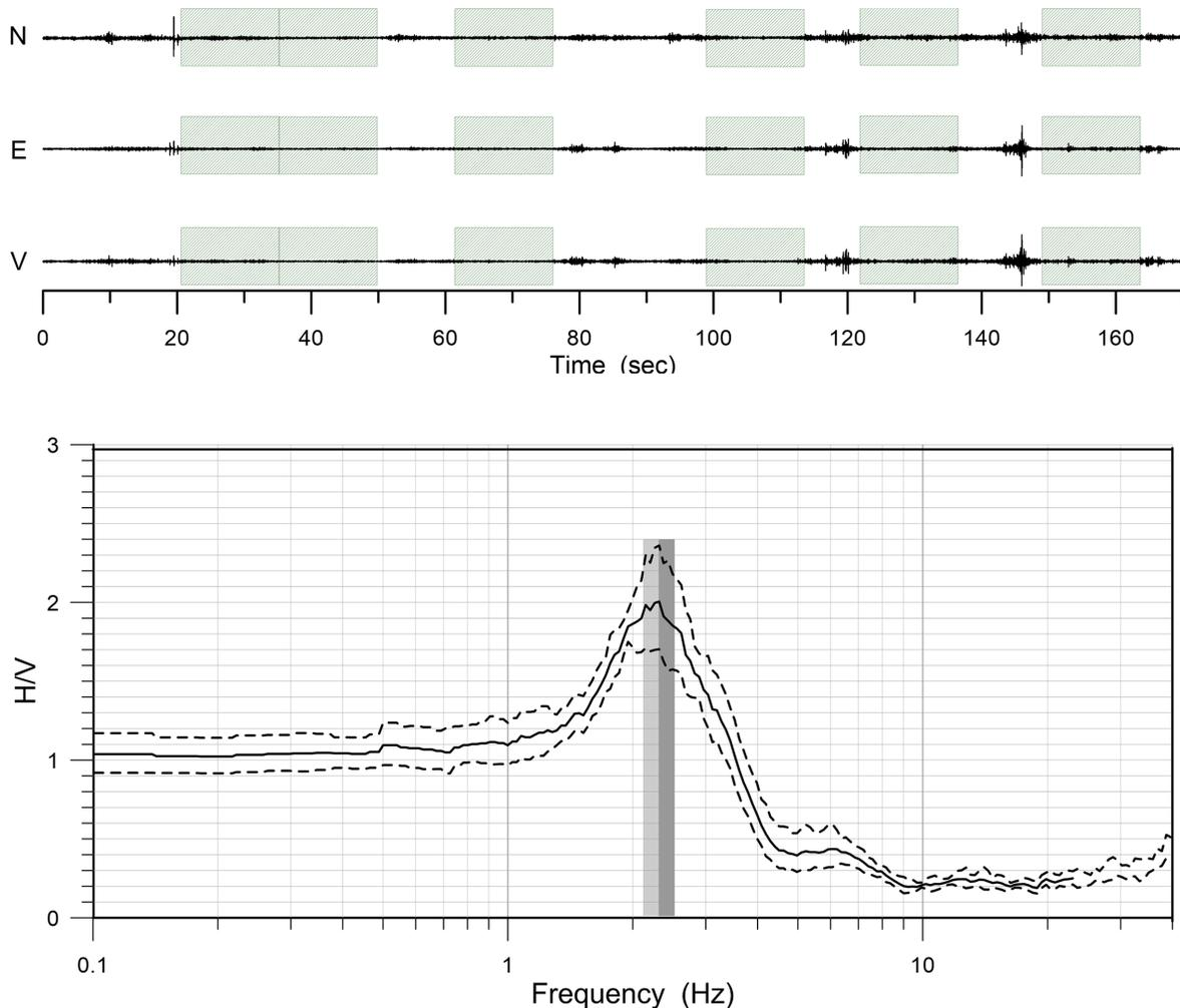
**Figure 9.** Example of a three component record (a) and spectral ratio (b) obtained at site P01. Green rectangles show the windows used. Shaded rectangles in (b) show the maximum amplitude. Dashed lines indicate standard deviation of the spectral ratios given by the different windows used.
