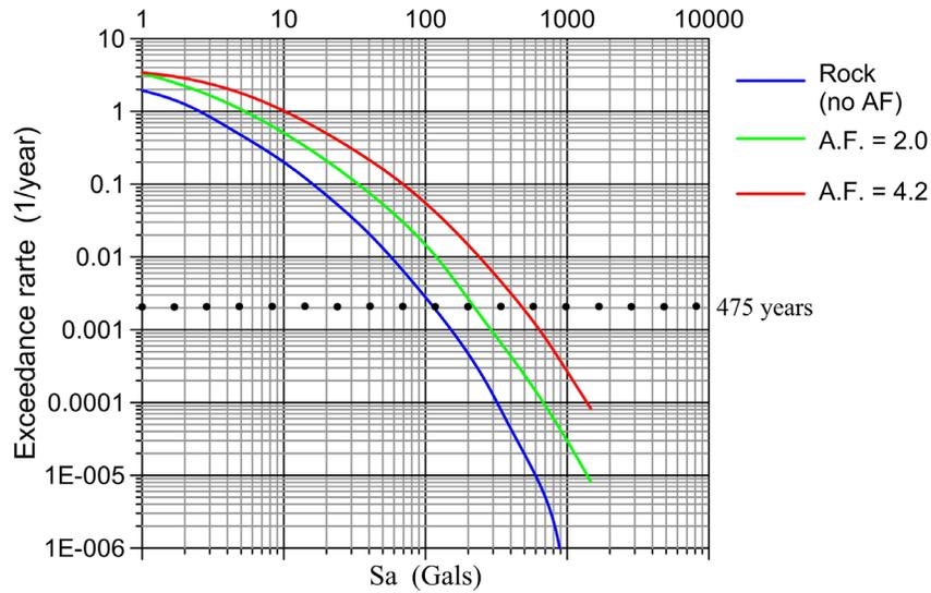
**Figure 11.** Seismic hazard curves for Los Mochis in terms of amplification factors.
