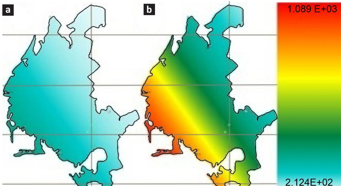
**Figure 12.** Seismic hazard map in terms of accelerations (gals). (a) for rock and (b) for soft ground considering 4.2 as amplification factor.
