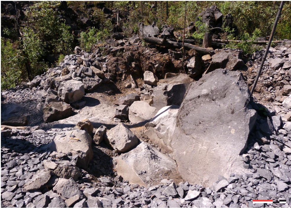
Figure 19. El Metate “El Cerro”: quarry of Don Pedro’s nephews, where the covering earth (humus) was removed prior to the breaking of the andesite blocks (Scale = 50cm).
