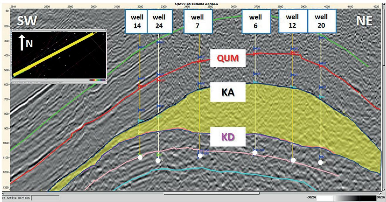
**Figure 10.** Seismic section shows the loss of seismic signal at large thicknesses of (KA) and the clarity degree of seismic signal at little thicknesses of (KA).
