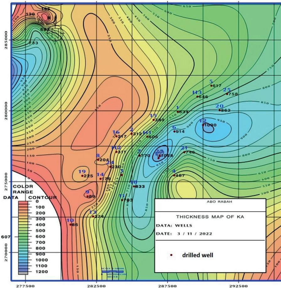
Figure 12. The thickness contour map of Kurachine Anhydrite (KA) formation in Abo-Rabah.
