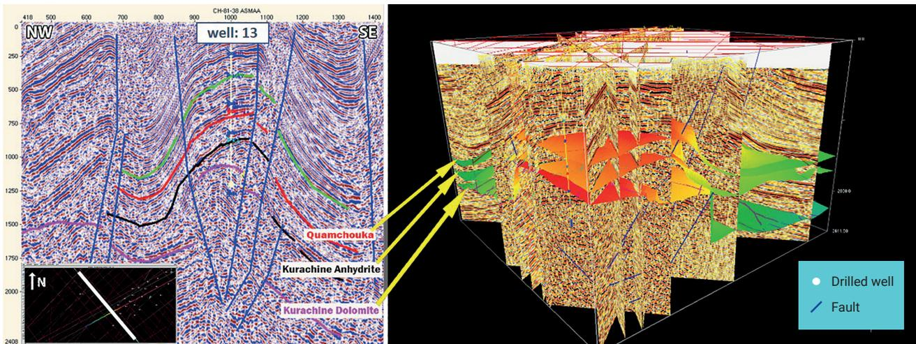
**Figure 8.** 3D representation of the 2D surveys with reflection surfaces and interpreted faults.
