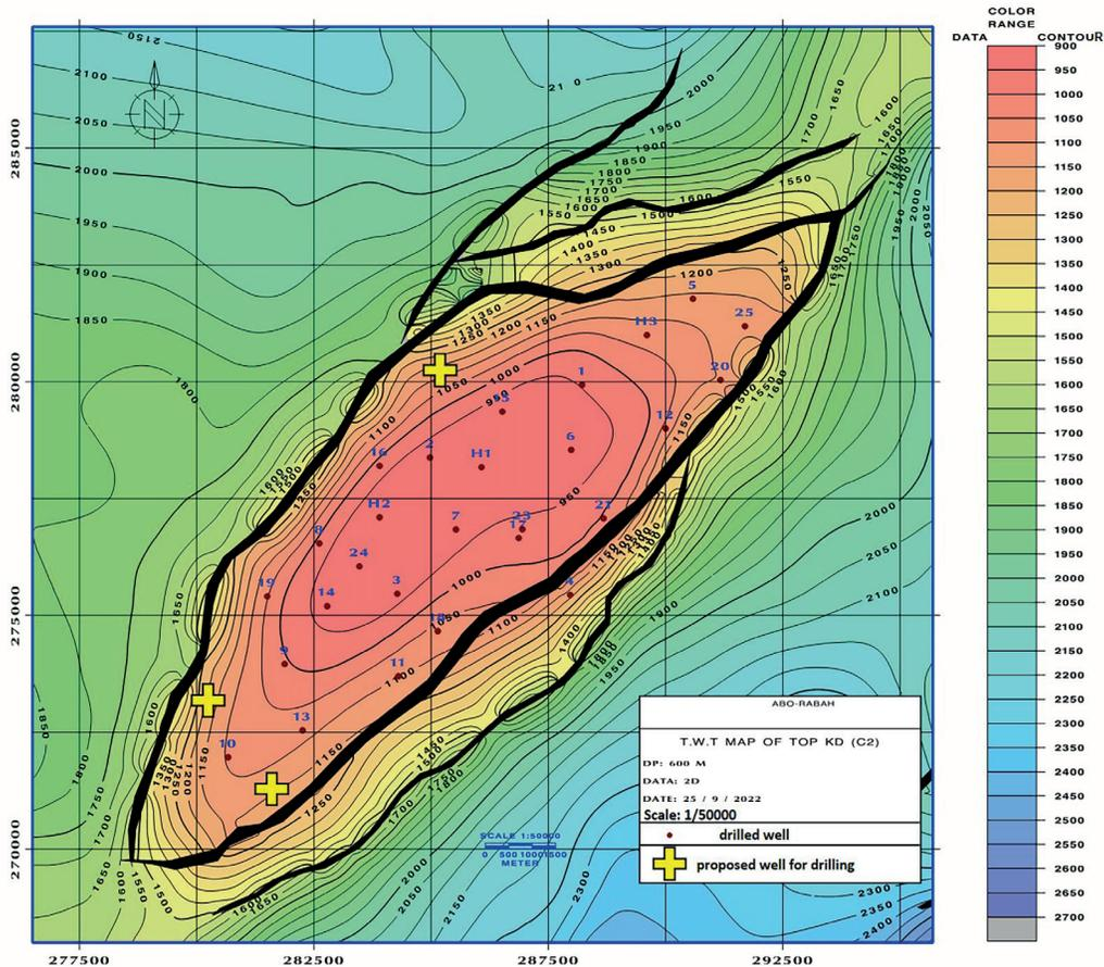
**Figure 14.** Time map (TWT) obtained for (KD) reflector in (Abo-Rabah) field and the chosen locations of boreholes proposed for drilling.
