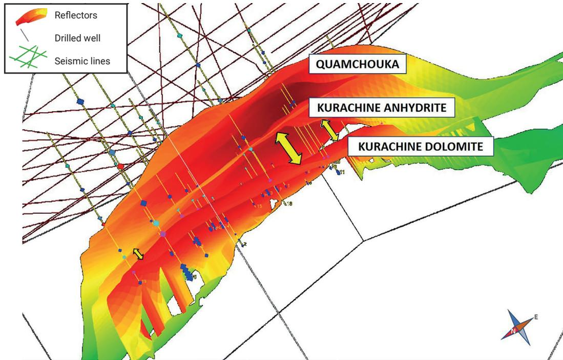
Figure 11. Three-dimensional section of the most significant reflectors in Abo-Rabah field.
