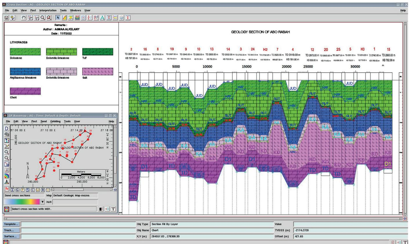
Figure 6. Correlation of litho-stratigraphic section passing through most of the wells in the Abo-Rabah area.
