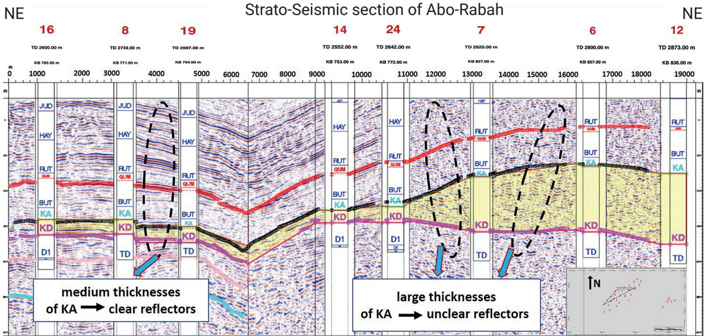
**Figure 13.** A strato-seismic section of the wells (16, 8, 19, 14, 24, 7, 6 and 12) in Abo-Rabah field, showing the blurring of the reflectors at the large thicknesses of the (KA), and their clarity when these thicknesses decrease.
