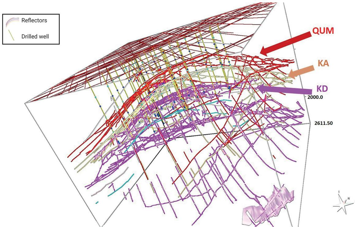
**Figure 7.** (3D) representation of interpreted reflectors, faults and fault profiles through (2D) lines in (Abo Rabah) area.
