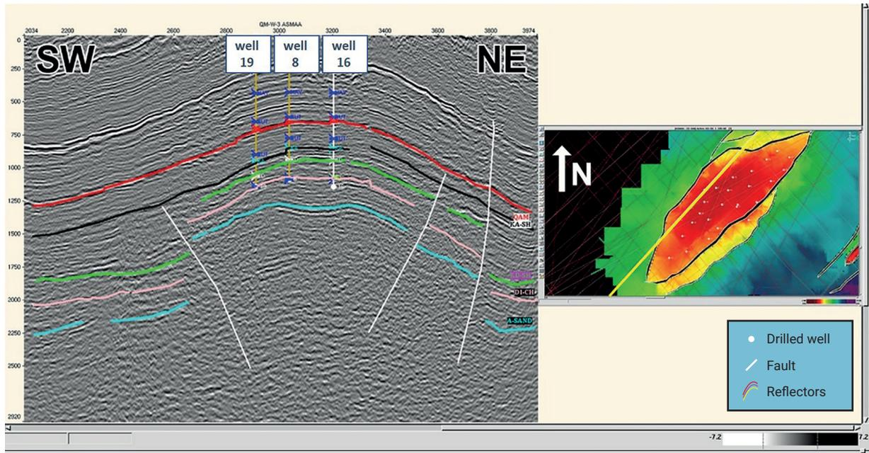
**Figure 9.** Seismic section prepared from processing data of QM survey lines in the study area.
