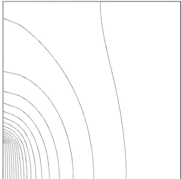
Fig. 2. Equidistant lines of equal head for the corner position of the filter and a near-square area.
