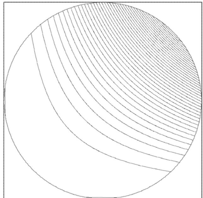
Fig. 5. Equidistant lines of equal head for a circular area.
