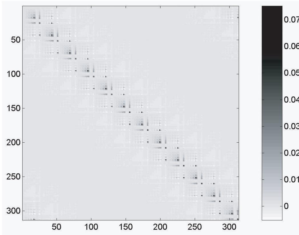
Fig. 4. Image of  $\mathbf{S}/\mathbf{S}$ .  $\mathbf{S}$  was assembled from the sensitivity maps calculated for a 12-electrode ECT sensor ( $m = 66$ ), with  $p = 313$ ,  $\epsilon_{\text{min}} = 1$  and  $\epsilon_{\text{max}} = 2.1$ .
