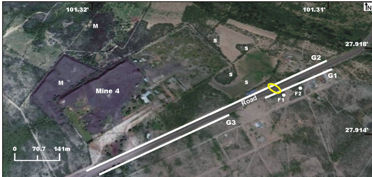
Figure 7. Study Sector 3. Continuous white lines indicate location of the measurement profile (G1, G2 and G3). S indicates areas with a sinkhole. F1 and F2 indicate the reference point for the photographs shown in figures 14c and 14d. Yellow ellipse indicates a subsidence zone on the road (view photography in Figure 14a).
