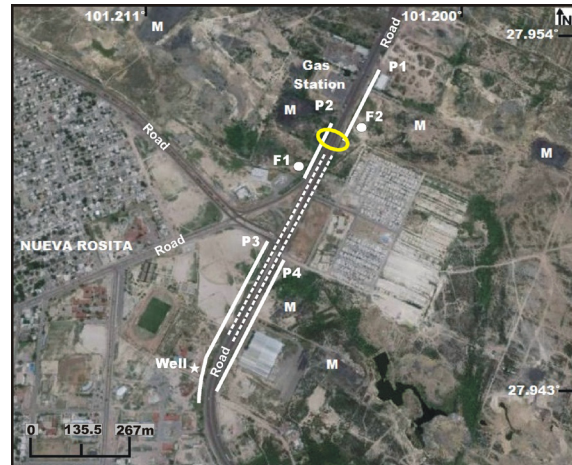
Figure 5. Study Sector 1. M indicates mining zones. Continuous black lines indicate location of the measurement profile (P1, P2, P3 and P4). Dashed black lines indicate location of the bridge. F1 and F2 indicate the reference point for the photographs shown in figures 9b and 9c. Yellow ellipse indicates a subsidence zone on the road (view photography in Figure 9a). Star indicates well.
