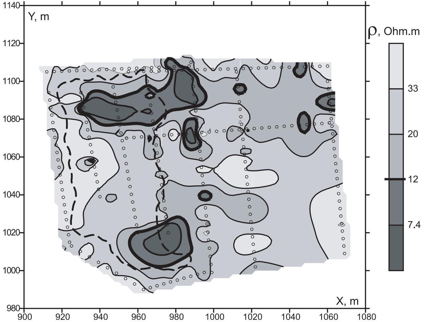
Fig. 5. Resistivity map for the optimal layer.
