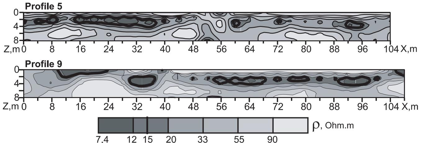
Fig. 4. Vertical resistivity cross-sections for profiles 5 and 9 after 2D interpretation with Res2DInv software.
