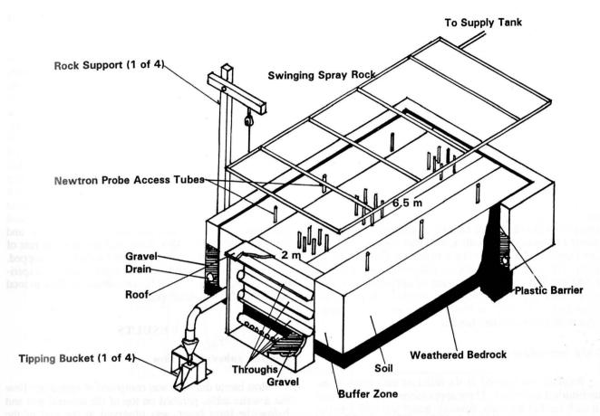
Fig. 1. Schematic drawing of the experimental layout and the soil block.
