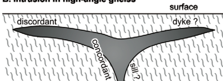
Fig. 9. Schematic diagrams for dyke-sill transition by mean of direction change of the \sigma_1 and \sigma_3 according to depth based on Hills (1975), in case of intrusion in: A) horizontal sedimentary formation; B) steeply dipped gneissic body.
