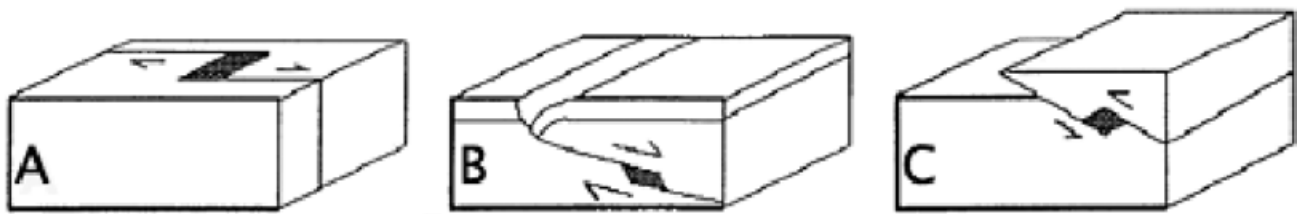
Fig. 4. Storage of evolved melt in releasing bends in different regional tectonic settings, Southwest Nevada Volcanic Field (modified from Cambray et al. , 1995). A) strike-slip, B) normal, C) reverse.
