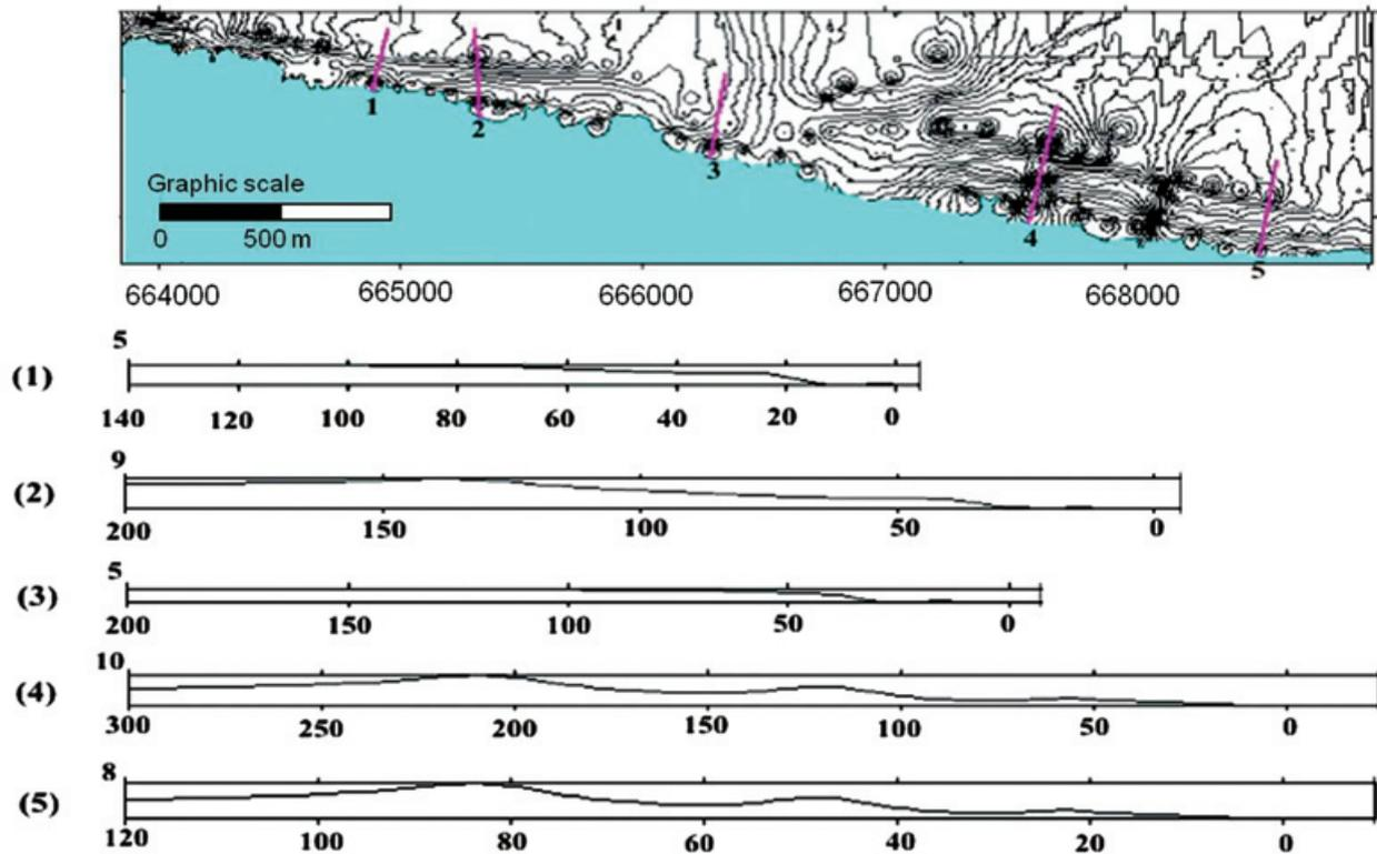
Fig. 7. Topographic map of Colola beach with profiles of topographic survey for Fall 1998.
