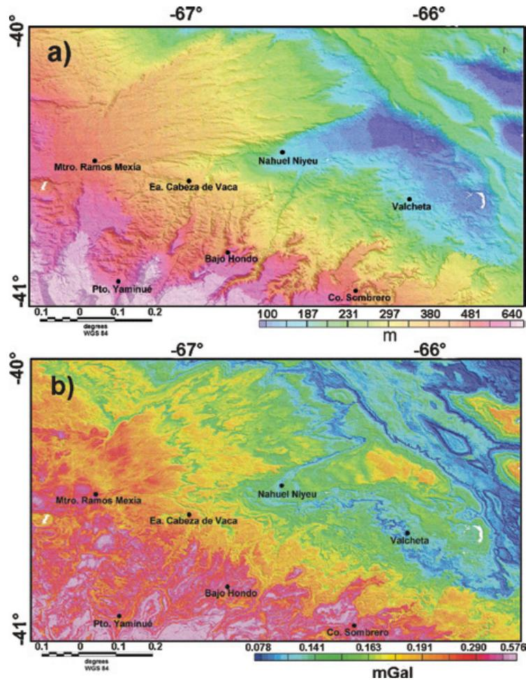
Fig. 2. a) a digital elevation model 90 m X 90 m. b) topographic correction- an internal radius of 90 m, external radius 167.000 m using a normal density of 2.67 g/cm<sup>3</sup>.
