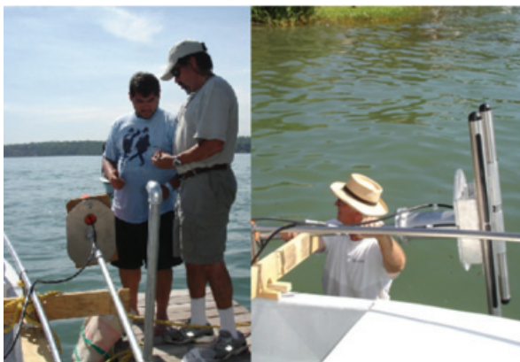
Figure 8. Photographs of the survey equipment. Left side, EA600 echosounder transducer. Right side, Sidescan sonar transducers.
