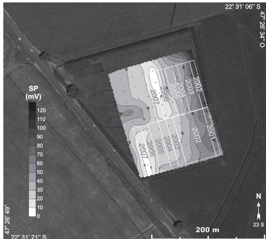
Figure 2. Self-potential map with closure ages of the ditches.
