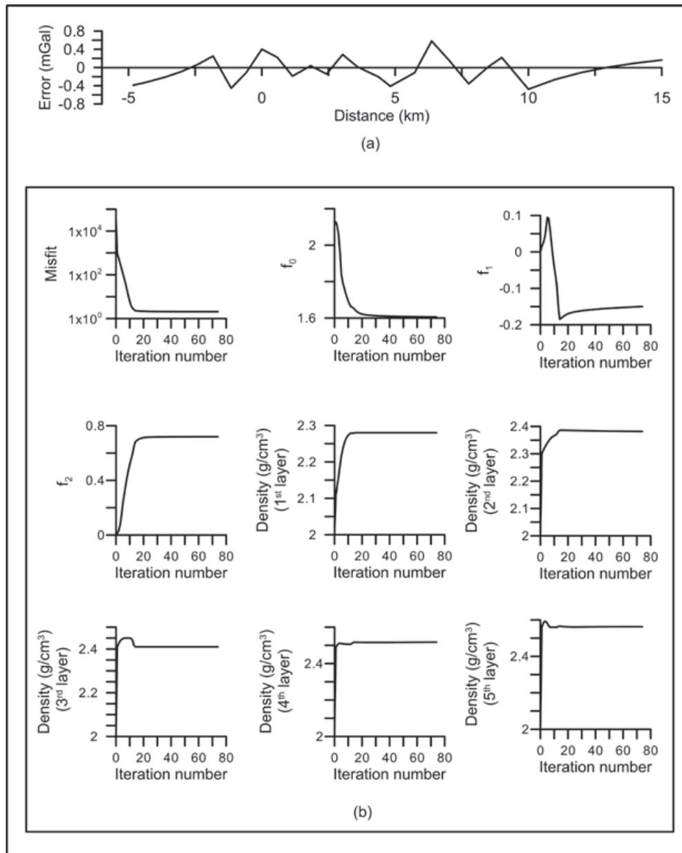
**Figure 10.** (a) Error analysis between the observed and modeled gravity anomalies across the Aswaraopet master fault, Chintalpudi subbasin, India, (b) changes in misfit, coefficients of a 2<sup>nd</sup> degree polynomial, and depths to various density interfaces against the iteration number.
