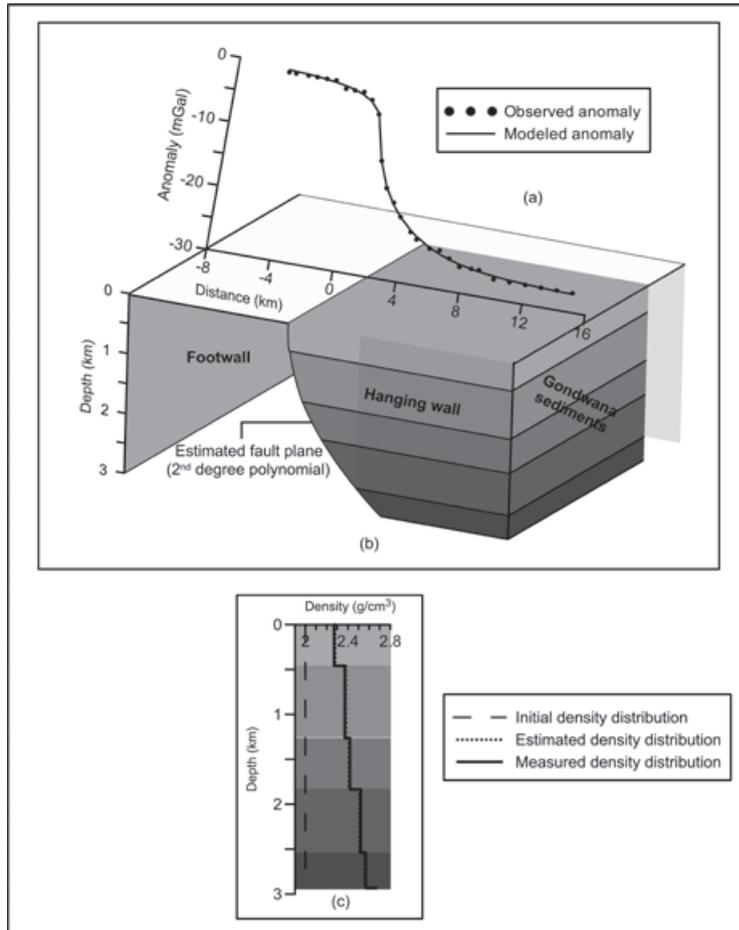
**Figure 7.** (a) Observed and modeled gravity anomalies, (b) inferred fault plane geometry of the Aswaraopet master fault, Chintalpudi subbasin, India, (c) assumed, initial and modeled densities. Depths of density interfaces are fixed during inversion.
