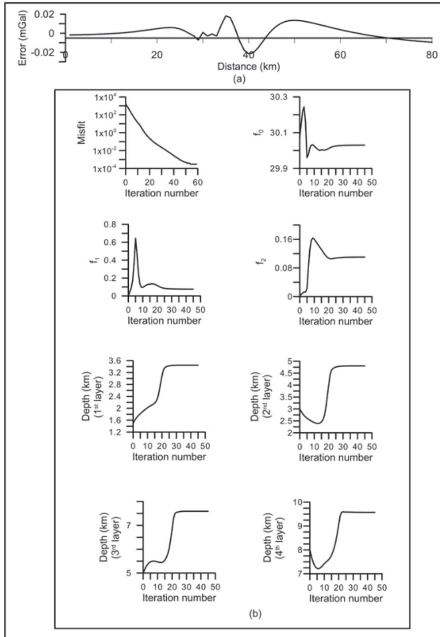
**Figure 5.** (a) Error analysis between the observed and modeled gravity anomalies, (b) changes in misfit, coefficients of a 2<sup>nd</sup> degree polynomial, and depths of various density interfaces against the iteration number.
