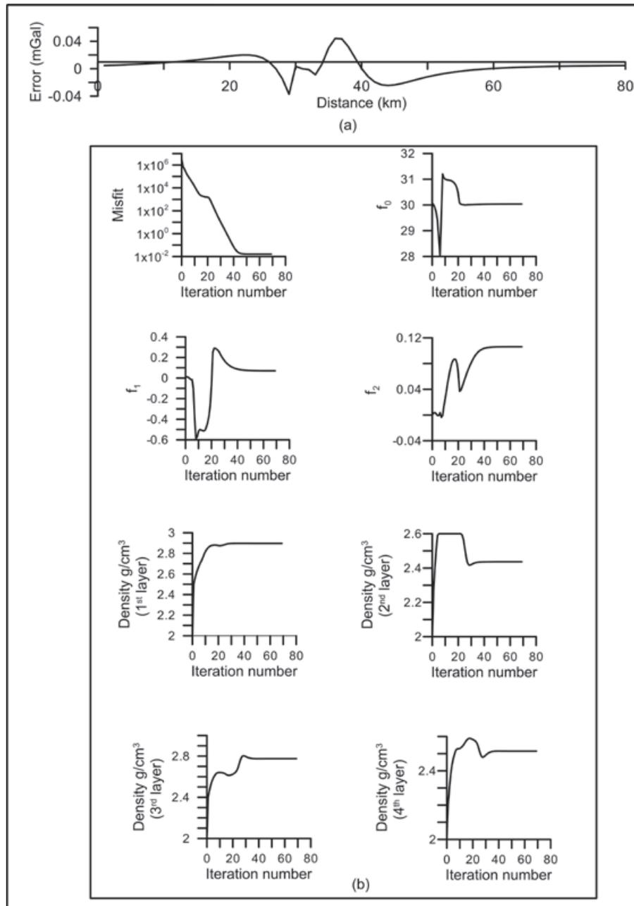
**Figure 3.** (a) Error analysis between the observed and modeled gravity anomalies, (b) Changes in misfit, coefficients of a 2<sup>nd</sup> degree polynomial, and densities of subsurface formations against the iteration number.
