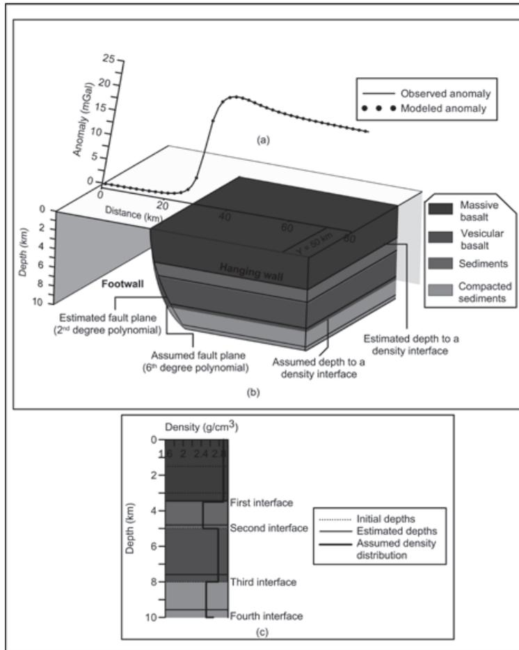
**Figure 4.** (a) Observed and modeled noisy gravity anomalies, (b) four layered hanging wall system of synthetic listric fault source with assumed and modeled fault planes described by 6<sup>th</sup> and 2<sup>nd</sup> degree polynomials, (c) assumed and estimated depths to density interfaces. Densities of the formations (shown as step line) are remain unchanged during inversion.
