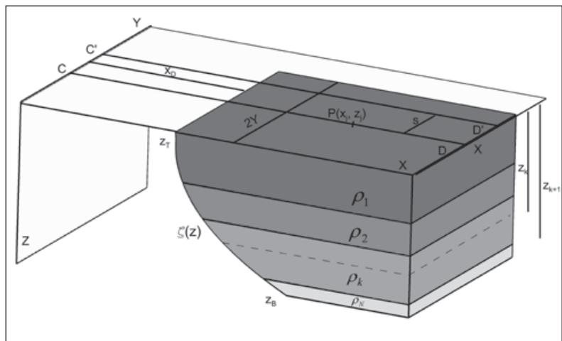
**Figure 1.** Schematic representation of a strike limited listric fault source. The detached downthrown block (hanging wall) is consisting of  $N$  horizontal formations with differing depths and densities. The limited strike length prevents the structure to represent as a 2D source.
