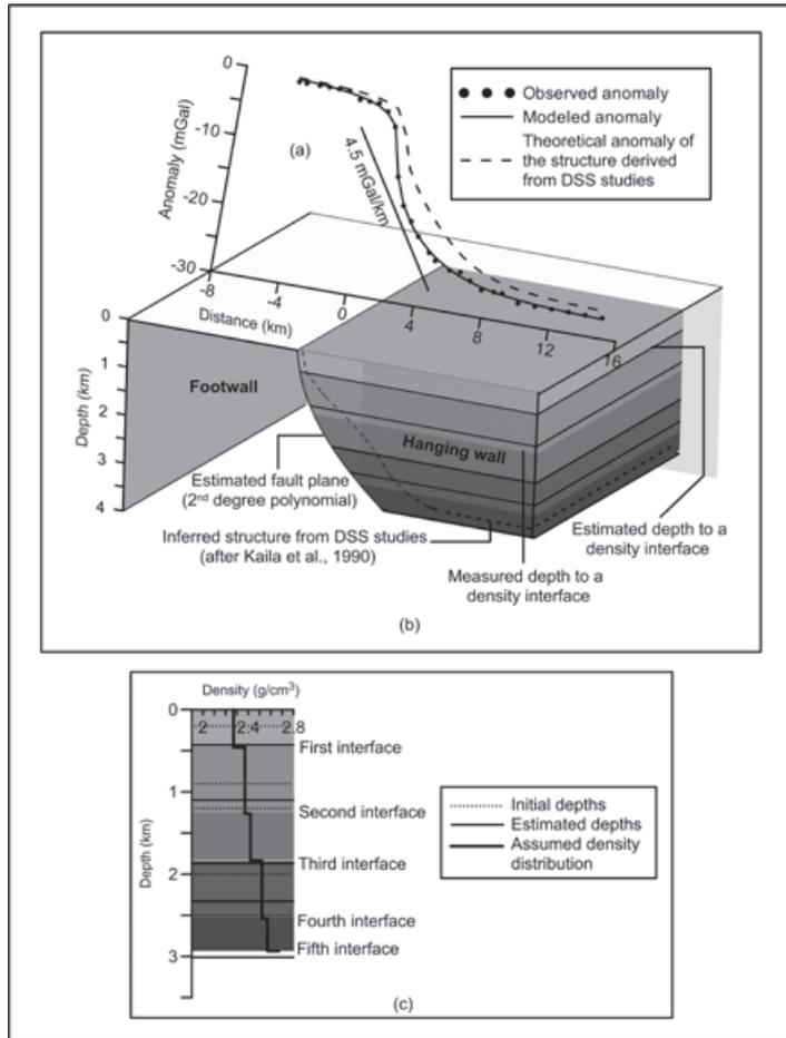
**Figure 9.** (a) Observed and modeled gravity anomalies, (b) inferred fault plane geometry of the Aswaraopet master fault, Chintalpudi subbasin, India. Anomalies are analyzed to estimate the depths of density interfaces.
