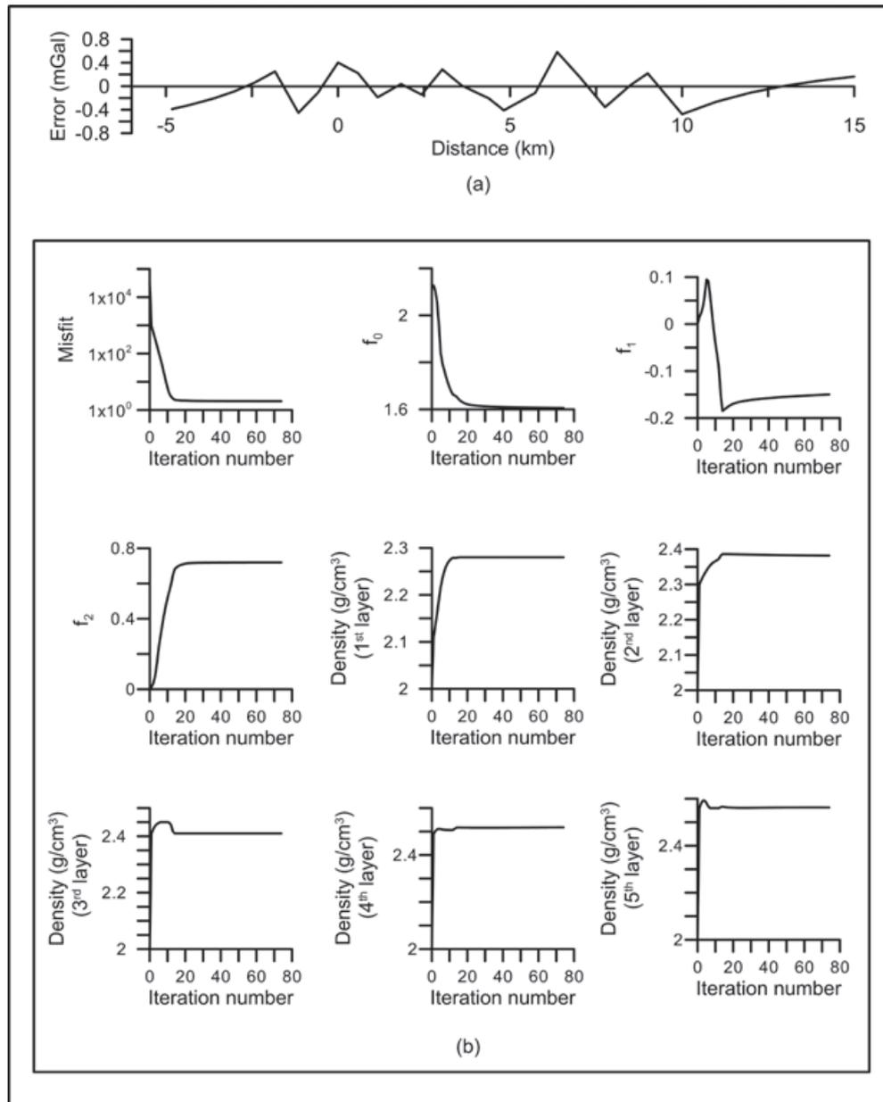
**Figure 8.** (a) Error analysis between the observed and modeled gravity anomalies across the Aswaraopet master fault, Chintalpudi subbasin, India, (b) Changes in misfit, coefficients of a 2<sup>nd</sup> degree polynomial, and densities of subsurface formations against the iteration number.
