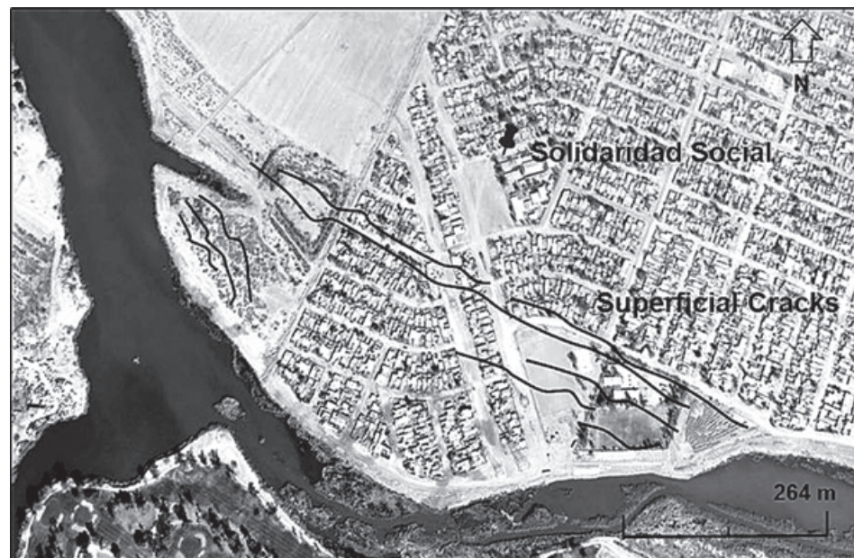
Figure 2. Superficial cracks and fractures.
