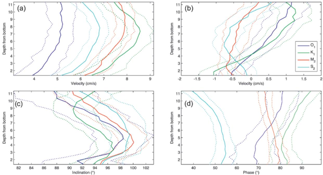
**Figure 4.** Vertical structure of the ellipse characteristics for the main tidal currents: (a) semimajor axis ( $\text{cm s}^{-1}$ ), (b) semiminor axis ( $\text{cm s}^{-1}$ ), (c) orientation of the semimajor axis, in degrees relative to East, positive counterclockwise, and (d) phase relative to tidal potential at Greenwich, in degrees. The dashed lines are the demarcation of the errors.
