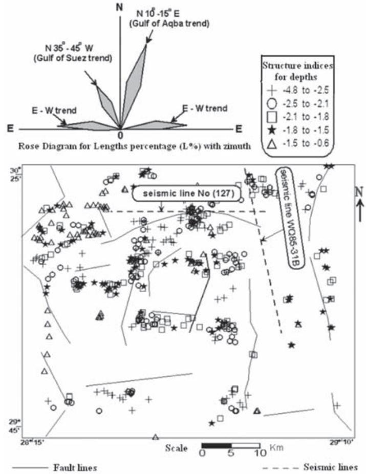
**Figure 12.** Fault structure lines as deduced from filtered magnetic anomaly maps.
