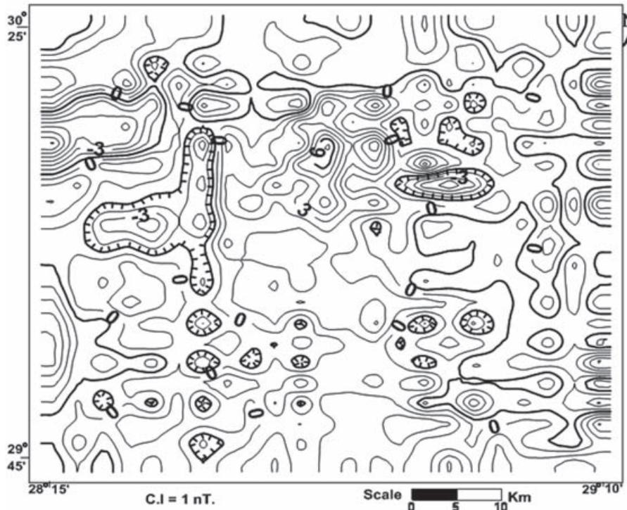
**Figure 7.** High-pass residual filtered aeromagnetic anomaly map.
