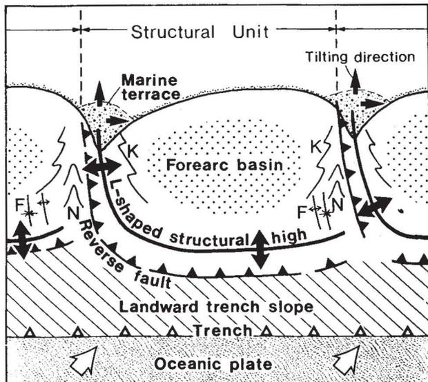
Fig. 10. Simplified topographic and structural features of the structural unit formed by the left-oblique subduction.
