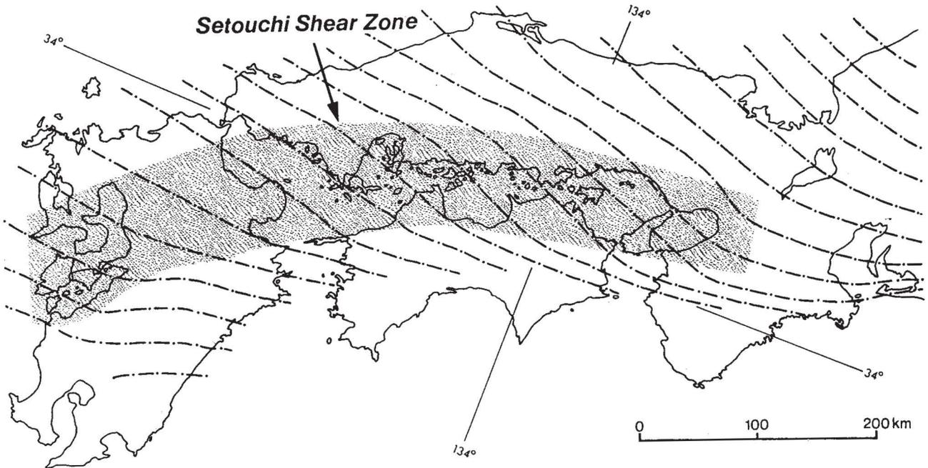
Fig. 16. Trajectories of maximum horizontal compressive stress obtained from focal mechanisms of crustal earthquakes. After Tsukuda(1992).
