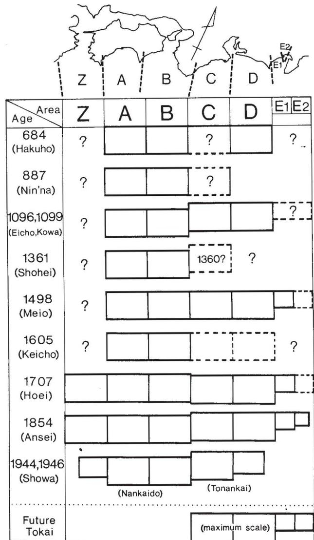
Fig. 11. Source areas of the successive plate-boundary earthquakes along the Nankai and Suruga Troughs. This figure was made on the basis of the reexamination of previous works on coseismic crustal movements, tsunami hazards and strong shaking caused by these earthquakes, from the viewpoint of structural unit model. Solid-line rectangles show probable ruptured areas (fault planes), and broken-line rectangles show uncertain ones.
