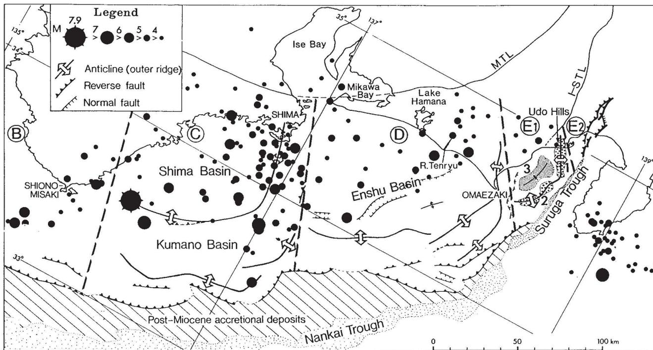
Fig. 12. Structural unit division of the off-Tokai region and epicentral distribution of earthquakes which occurred within 30 days after the 1944 Tonankai earthquake. After Sugiyama (1990). The location of epicenters is after Iwata and Hamada (1986). The topographic features in the unit E1 are 1: Kuno spur, 2: north and south Senoumi banks, and 3: Senoumi basin.
