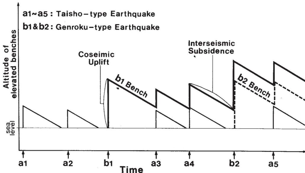
Fig. 8. Schematic formation model of elevated benches by coseismic uplifts associated with the Genroku-type earthquakes.
