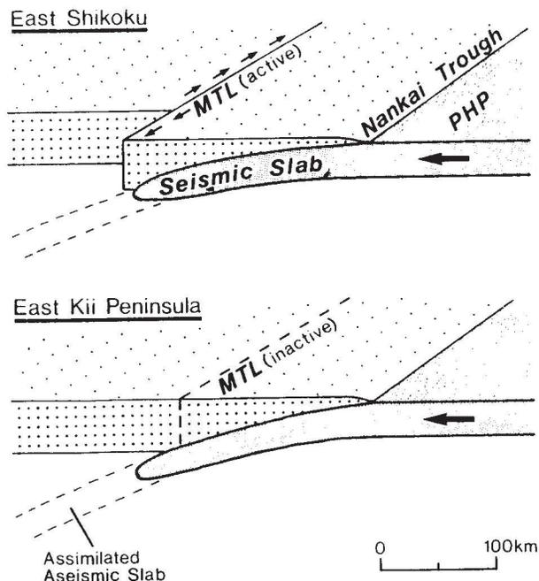
Fig. 21. Schematic figure showing the positional relation of leading edges of the seismic slab to the Median Tectonic Line in east Shikoku and east Kii Peninsula. Modified after Shiono(1992).
