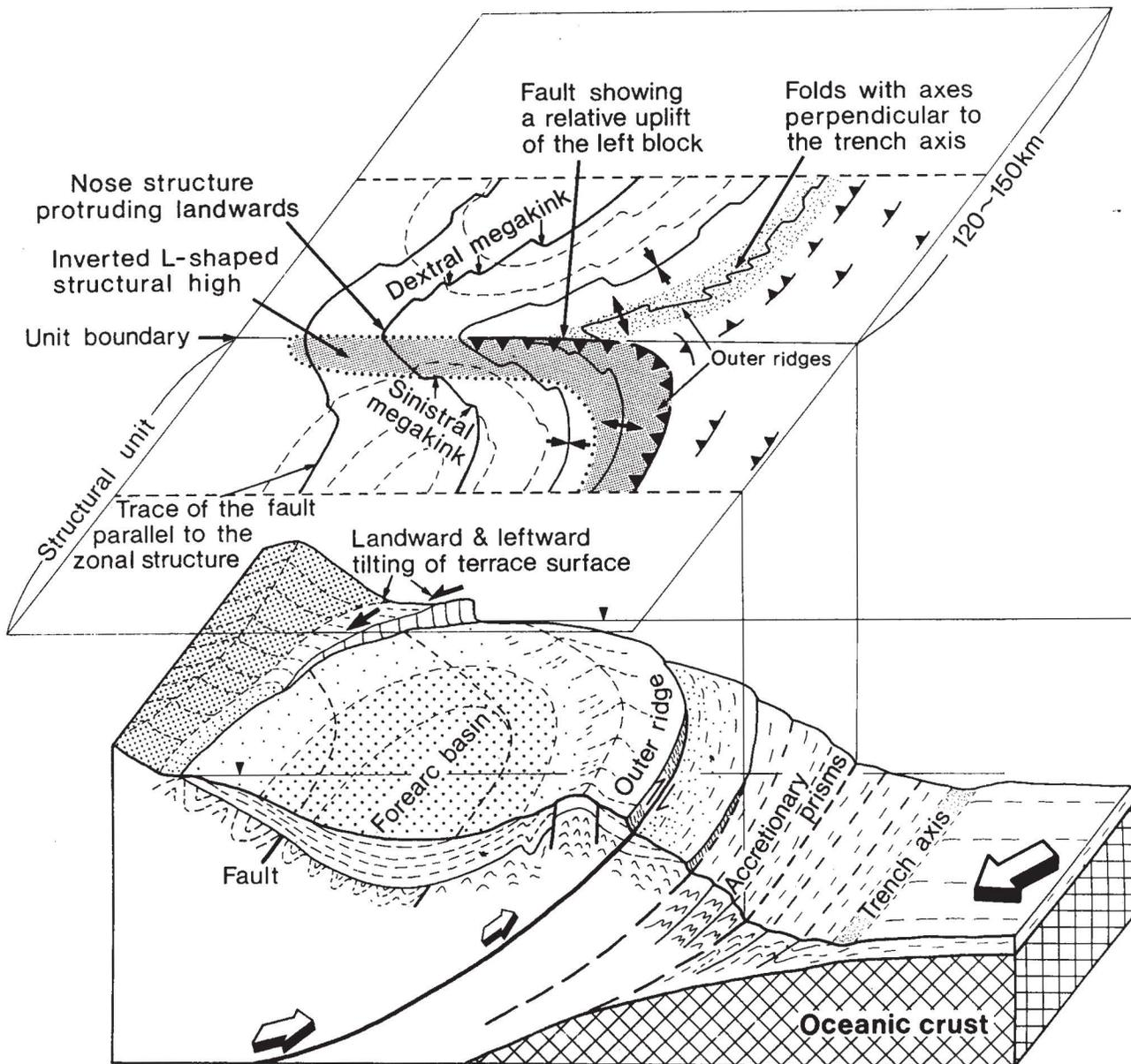
Fig. 9. Generalized formation model of topographic and structural features of the structural units formed by the right-oblique subduction. Modified after Sugiyama(1989).
