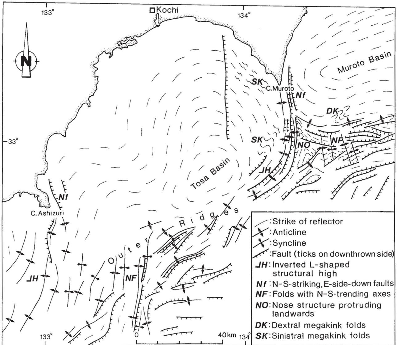
Fig. 4. Detailed geologic structures off Shikoku revealed by seismic profiling. Simplified after Okamura and Joshima (1986) and Okamura *et al.* (1987).
