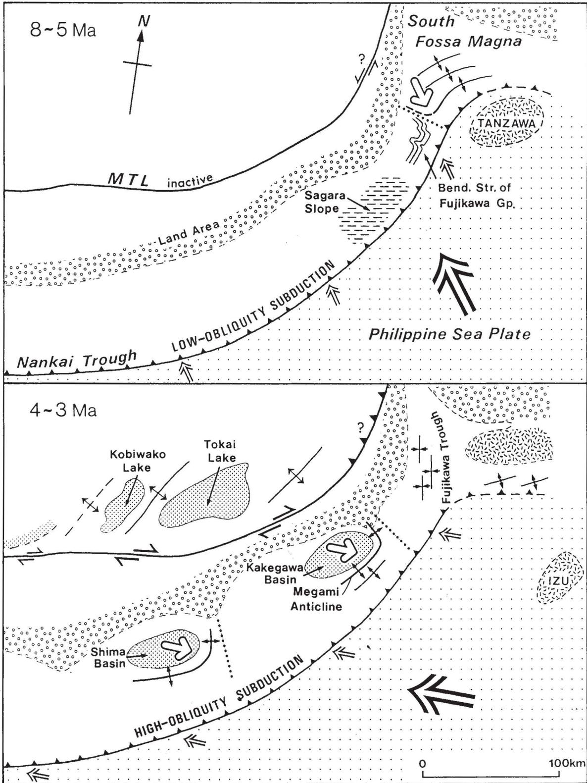
Fig. 20. Possible formation model of structural units in the forearc region and en-echelon basins along the MTL in relation to the initiation of right-oblique subduction of the Philippine Sea plate along the Nankai Trough. After Sugiyama(1991). Arrows in the South Fossa Magna (top figure) and in the Kakegawa and Shima basins (bottom figure) show the displacement direction of hanging walls of the causative faults of plate-boundary earthquakes.
