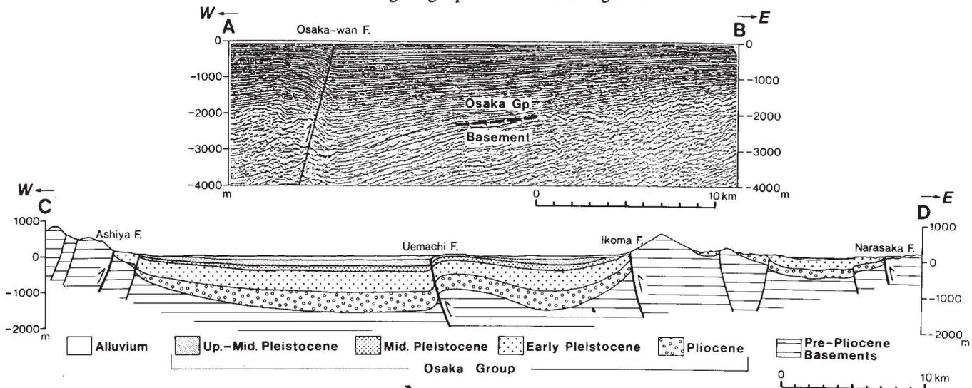
Fig. 15. Multichannel seismic reflection profile of Osaka Bay(A-B) and geologic profile of the Osaka area(C-D). The seismic reflection profile is after Iwasaki *et al.* (1990). The geologic profile of the Osaka area is after Itihara *et al.*(1991). See Figure14 for the locations of lines A-B and C-D.
