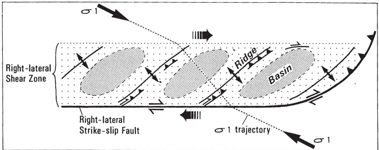
Fig. 17. Schematic formation model of right-handed en-echelon basins and ridges along a major right-lateral strike-slip fault. After Sugiyama(1991).
