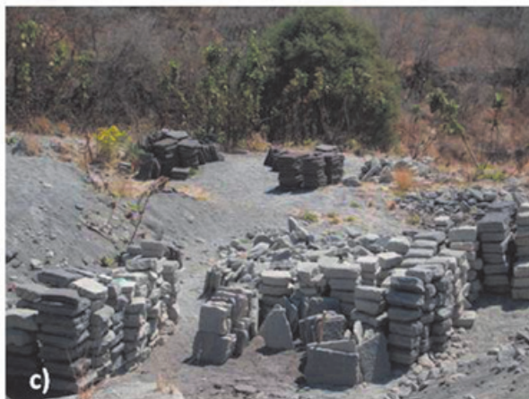
Figure 5. Views of the Xalnene tuff. (a) View of the quarry zone investigated by the resistivity soundings. (b, c) Views of the quarry operations, showing the trenches and the slabs cut from the ash layers. (d) View of marks left from quarry operations, modified by erosion. (a) View of marks produced by the mechanical excavator, partly eroded. The incision pattern with parallel groves can be observed.
