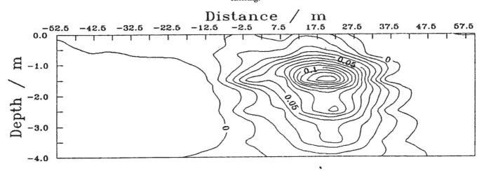
Fig. 5. Inversion of real magnetic data (see Fig. 4) using weighted minimum length inversion in the frequency domain. The map shows the computed distribution of susceptibilities within the model.
