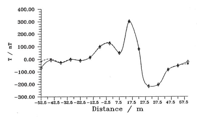
Fig. 4. Total magnetic field anomaly over a filled pit (solid line: measured anomaly, dashed line: computed anomaly). The computed anomaly differs at both edges slightly from the measured anomaly due to edge effects inherent in the numerical realization of inverse linear filtering.
