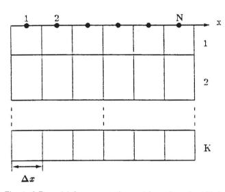
Fig. 1. 2-D model for computation and inversion of gridded potential field data (• denotes nodes of the grid).
