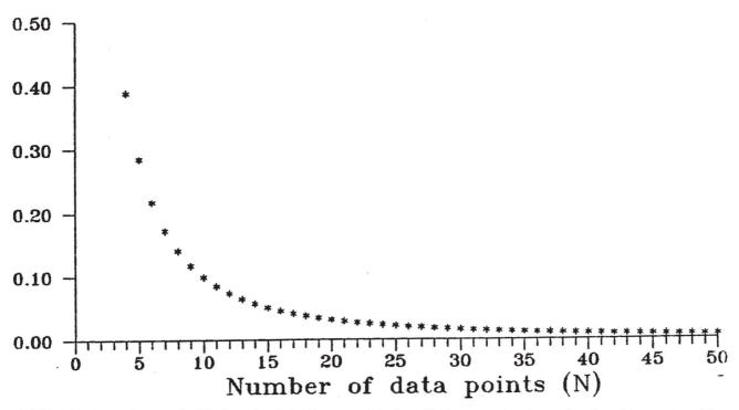
Fig. 6. Ratio of operations required for inversion in the frequency domain and in the space domain as a function of the number of data points N. The number of layers is set to K = 10.
