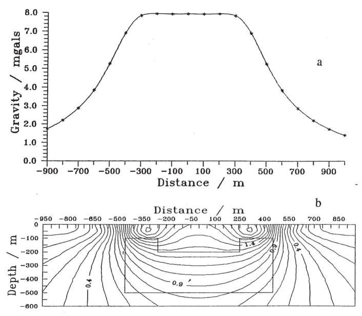
Fig. 2. Inversion of gravity data using minimum length inversion in the frequency domain. (a) gravitational attraction of the model; (b) synthetic model in comparison with the result of inversion.
