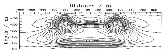
Fig. 3. Inversion of gravity data using weighted minimum length inversion in the frequency domain. A much improved correlation between synthetic model and computed density distribution is achieved.
