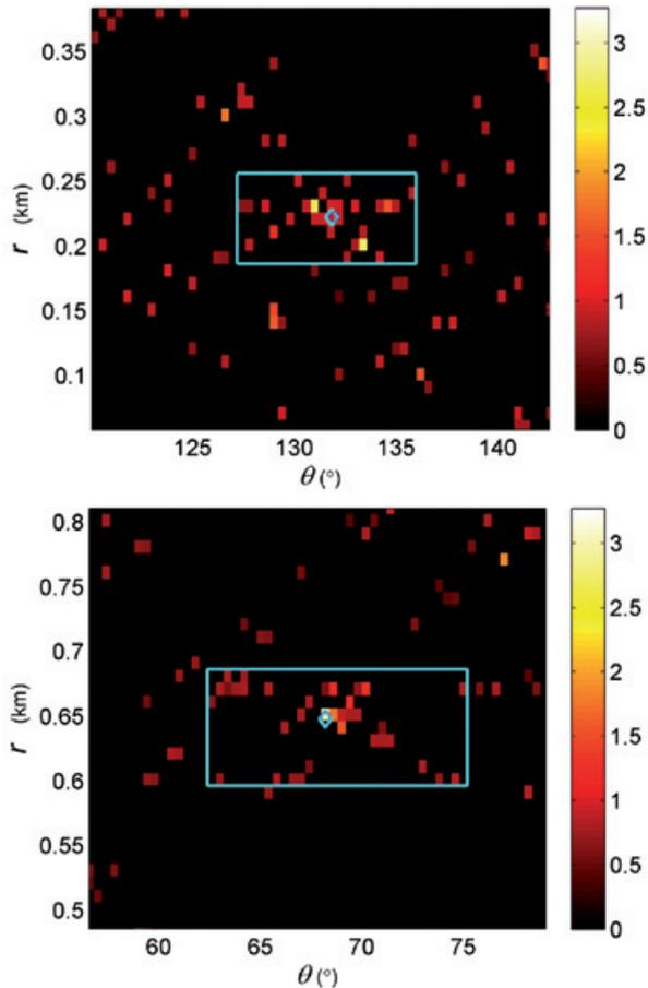
**Figure 8.** Close-up of the accumulator cells used for determining the values of the parameters of lines 1 (top) and 2 (bottom). The rectangles contained the cells used, the determinations are shown as diamonds, and the true values are indicated by circles
