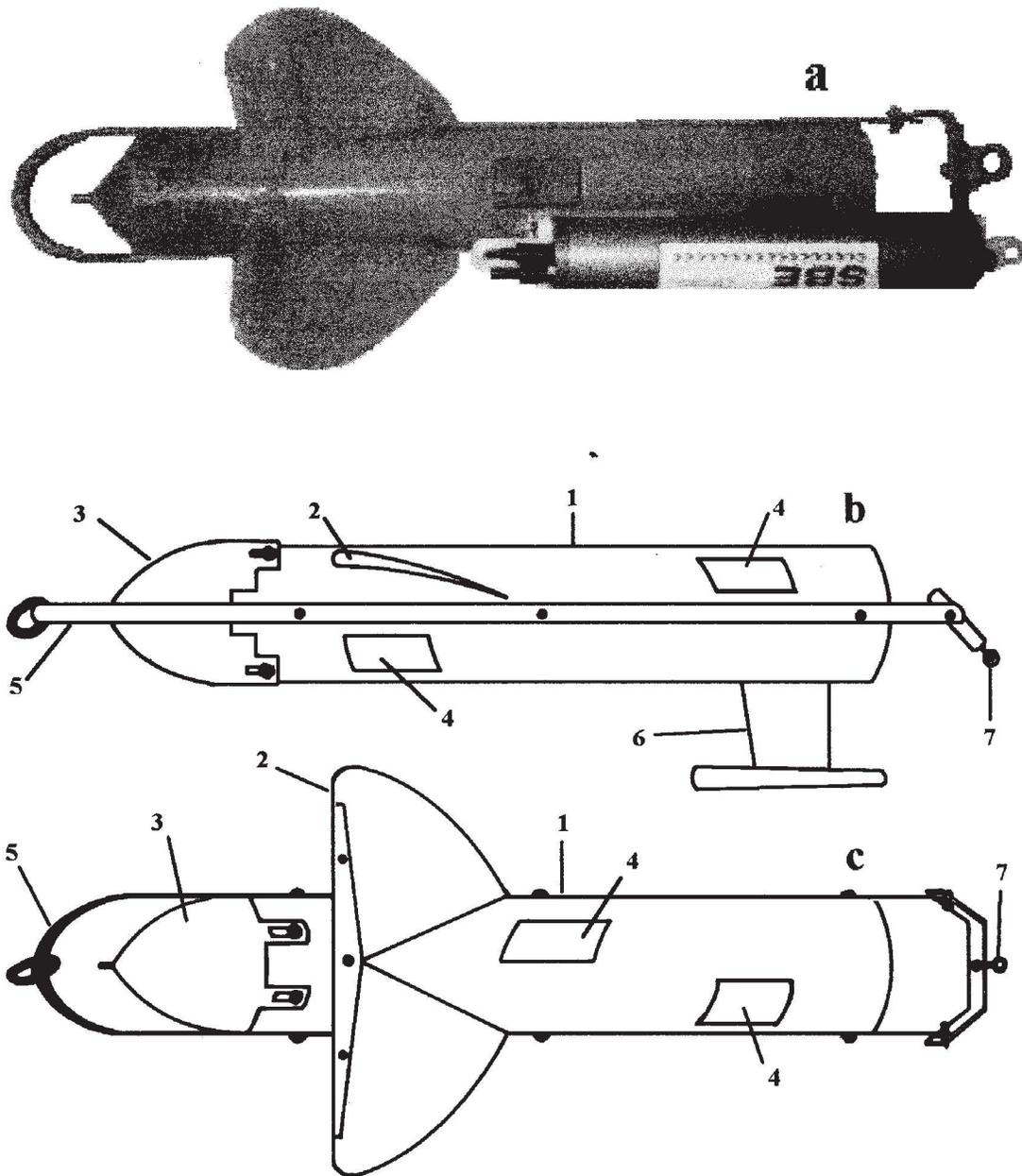
Fig. 1. (a) Towing case and CTD recorder. Figures (b) and (c) show lateral and top views. 1- Case. 2- Fins for sustentation, which provide a positive buoyancy while being towed. 3- Hydrodynamic removable lid. 4- Openings to allow flow of water through the case while it sinks. 5- Steel bar around the case for towing. 6- Directional keel to avoid rotation while towing. 7- Steel structure for attaching additional weights in order to regulate the speed of descent.
