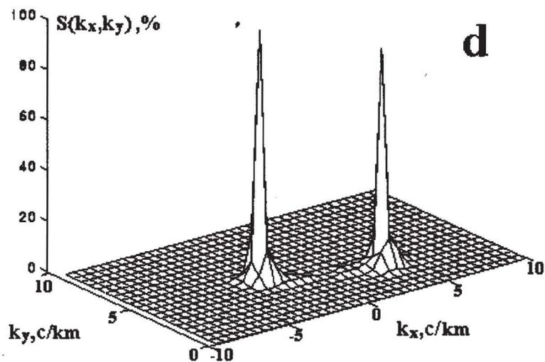
Fig. 4. (a) Spectral window based on the spatial position of the last seven stations of the micropolygon. Estimated average spatial spectra for temperature fluctuations at the stations, calculated using (b) the linear method, (c) the Maximum-Likelihood method, and (d) the Maximum-Entropy method. The spectral density profile is given as the ratio of the percentage to the maximum value.
