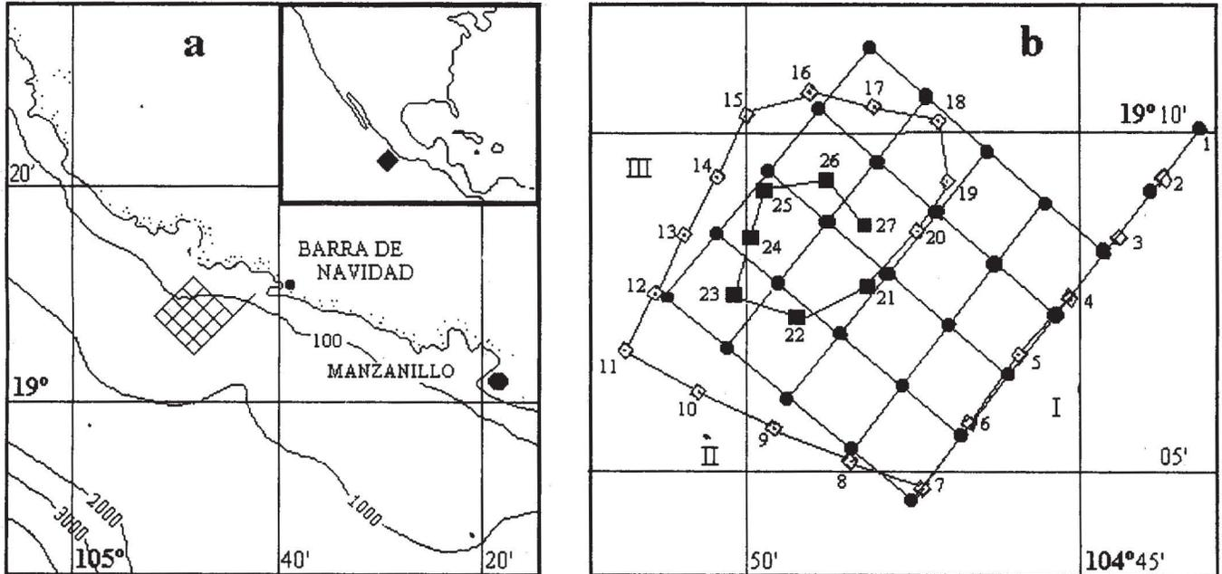
Fig. 2. (a) Micropolygon in which the fast-surveying method was tested. (b) Planned stations (solid dots) and actual positions of stations (squares) in the micropolygon. The transects are labeled with Roman numerals.
