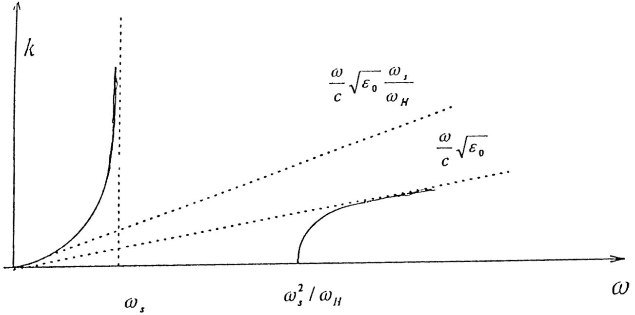
Fig. 2. Low-frequency electromagnetic waves for angle  $\theta = \pi/2$ . In the frequency range  $0 \leq \omega < \omega_s$  the wave is slow; in the frequency range  $\omega \geq \omega_s^2 / \omega_H$  the wave is fast.
