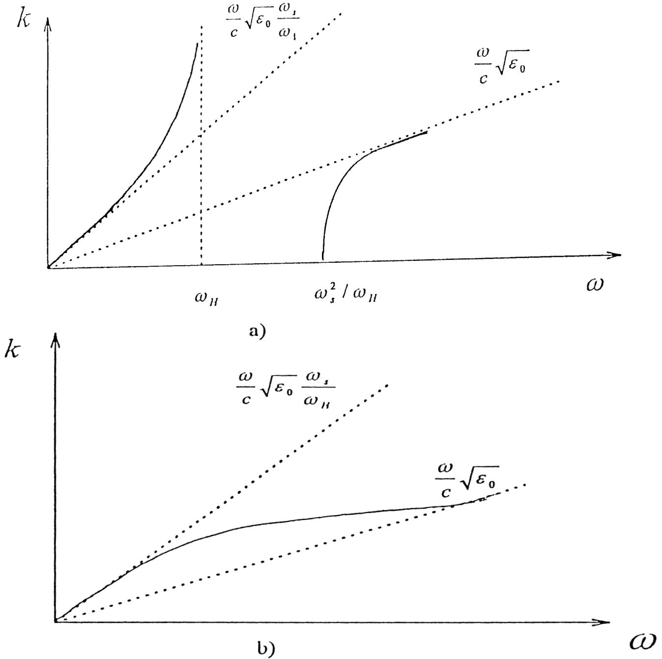
Fig. 1. Low frequency electromagnetic waves for the angle  $\theta = 0$ . (a) Left-rotating: in frequency ranges  $0 \leq \omega < \omega_H$  the wave is slow; in the frequency range  $\omega \geq \omega_s^2 / \omega_H$  the wave is fast; (b) right rotating: the wave exists in frequency range  $0 < \omega < \infty$ .
