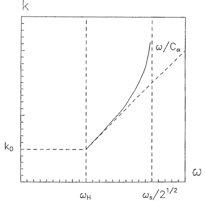
Fig. 4. Dependence  $k(\omega)$  for the surface wave in the case  $\vec{B}_0 \parallel \vec{k}$ .
