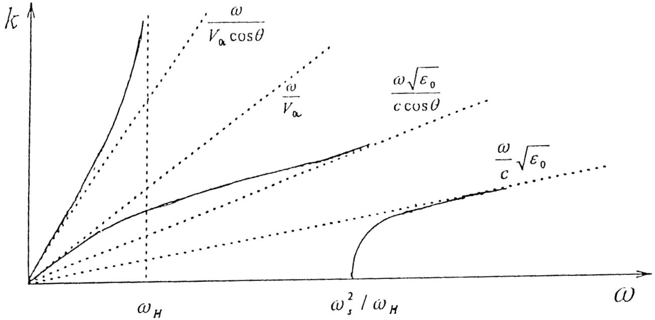
Fig. 3. Alfvén and magnetoacoustic waves.
