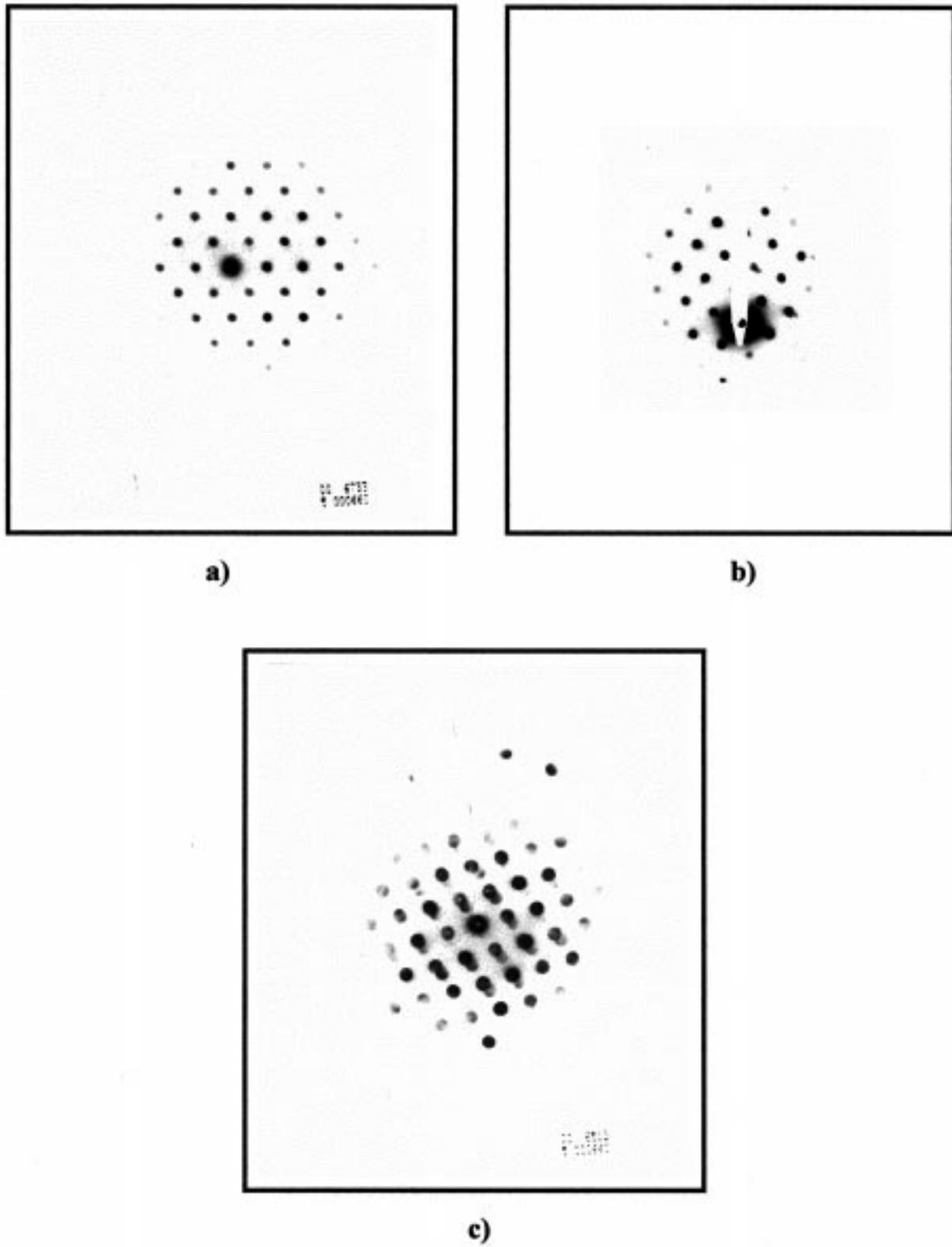
Fig. 7. Characteristic diffraction patterns (Transmission Electronic Microscopy by X-ray energy dispersion) obtained for magnetic separates corresponding to levels of high  $MS/|M|$  values. These patterns reveal the presence of magnetite (face centered cubic crystal) with  $d_o = 8.32\text{\AA}$  for LVT-4X (a),  $d_o = 8.37\text{\AA}$  for LVT-1X (b), and  $d_o = 8.25\text{\AA}$  for LVT-2X (c).
