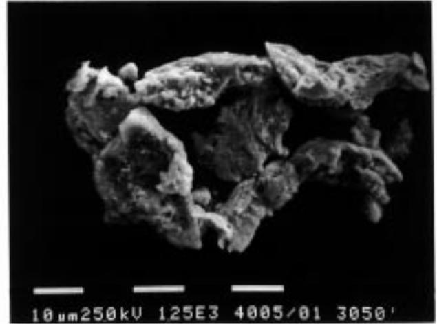
Fig. 6. Scanning electron photomicrograph (topographic image of secondary electrons) of a non-spherical aggregate of Fe-rich submicronic magnetic minerals (as found from X-ray energy dispersion spectra). This sample comes from a magnetic separate of a level with low MS and |M| values (LVT-4X; 915-930 depth interval).
