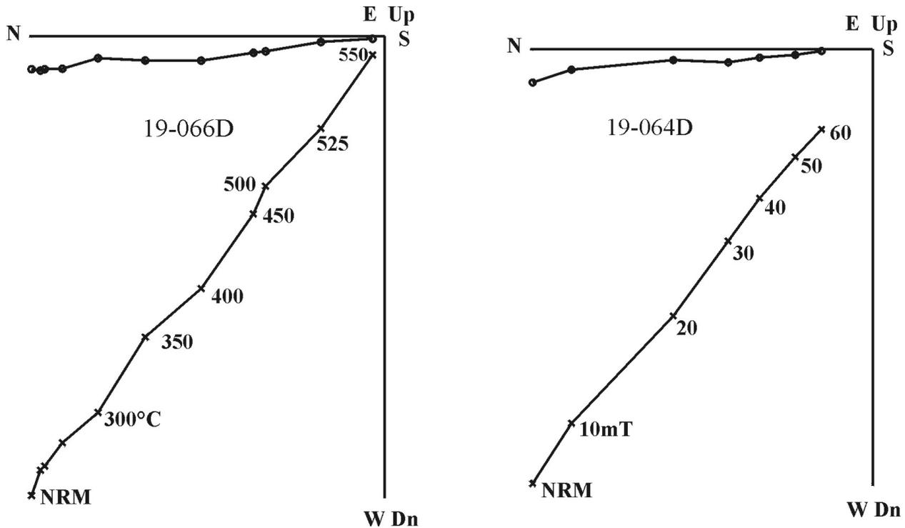
Fig. 1. Orthogonal vector plots of stepwise thermal or alternating field demagnetisation of selected samples. The numbers refer either to temperatures in °C or to peak alternating fields in mT. o – projections into the horizontal plane, x – projections into the vertical plane.
