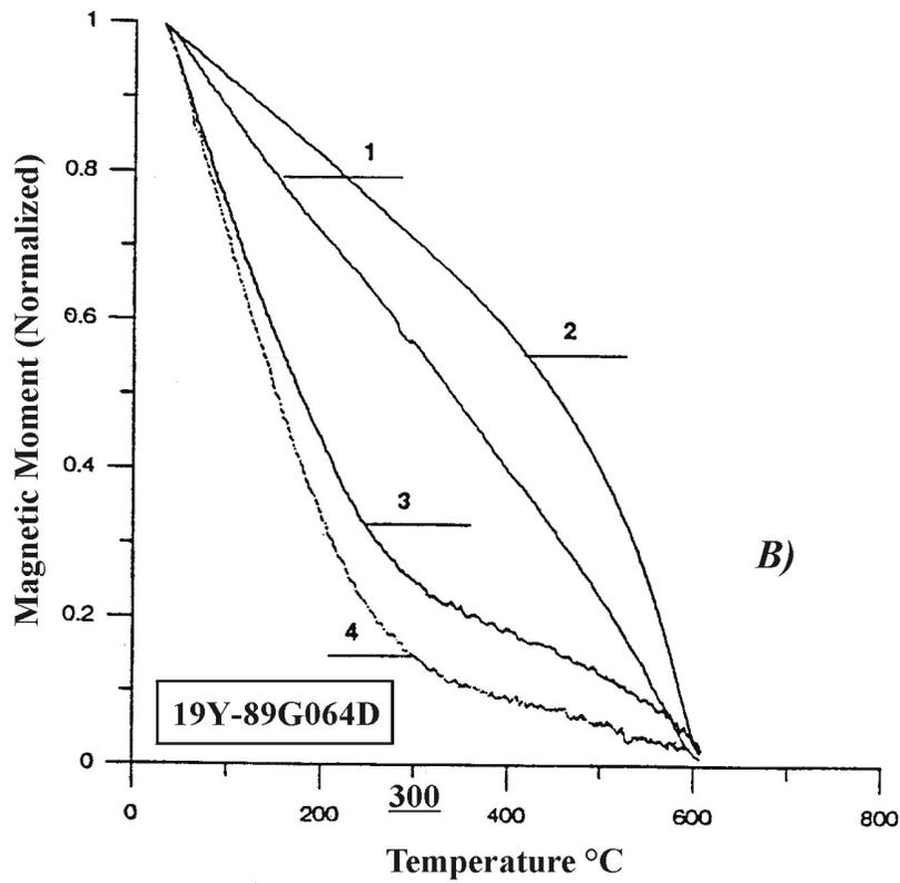
Fig. 4. Notation as in Figure 1. Curve 4 is a continuous thermal demagnetization of partial thermoremanence acquired in a field of 50  $\mu$ T, from 300°C to room temperature after treatment with liquid nitrogen (See also text).
