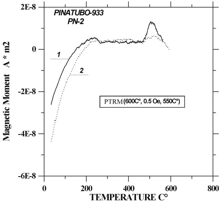
Fig. 5. Continuous thermal demagnetization of partial thermoremanence acquired in a field of 50 μT, cooling down from 600°C to 550°C before (curve 1) and after (curve 2) LTD treatment (see also text).
