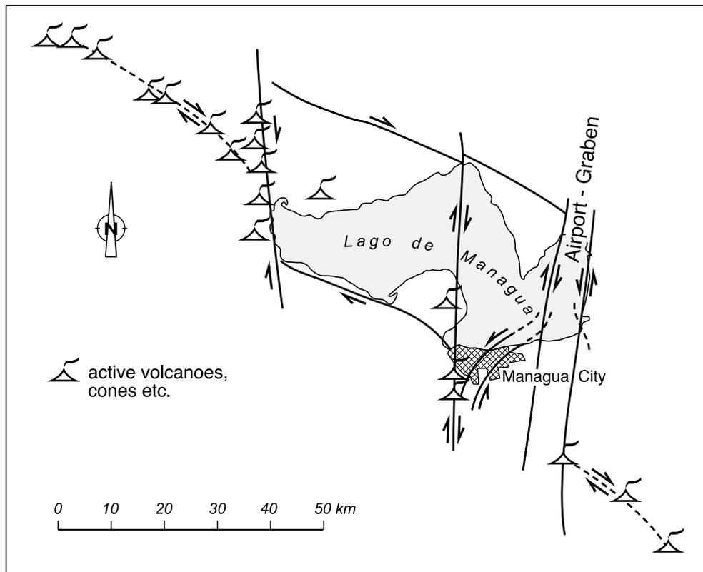
Fig. 11. Combined kinematic model for the Managua Fault Zone. The internal structure of the marginal zones of the Airport graben is indicated with broken lines.
