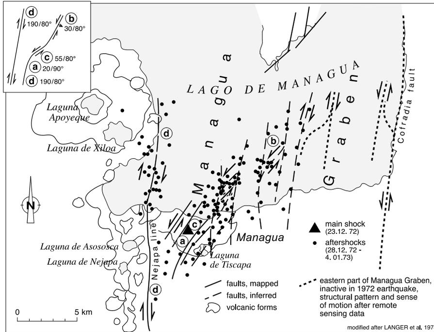
Fig. 9a. The activated fault pattern and aftershock distribution for the 1972 Managua earthquake is shown, completed within the eastern part of the structure after results of remote sensing interpretations. The letters (a) to (d) refer to results of fault plane solutions after BROWN *et al.* (1973). The inset map shows their transformation (cf. Fig.10) in a sketch map (compare the aftershock distribution (Fig. 9b) by WARD *et al.*, 1973).
