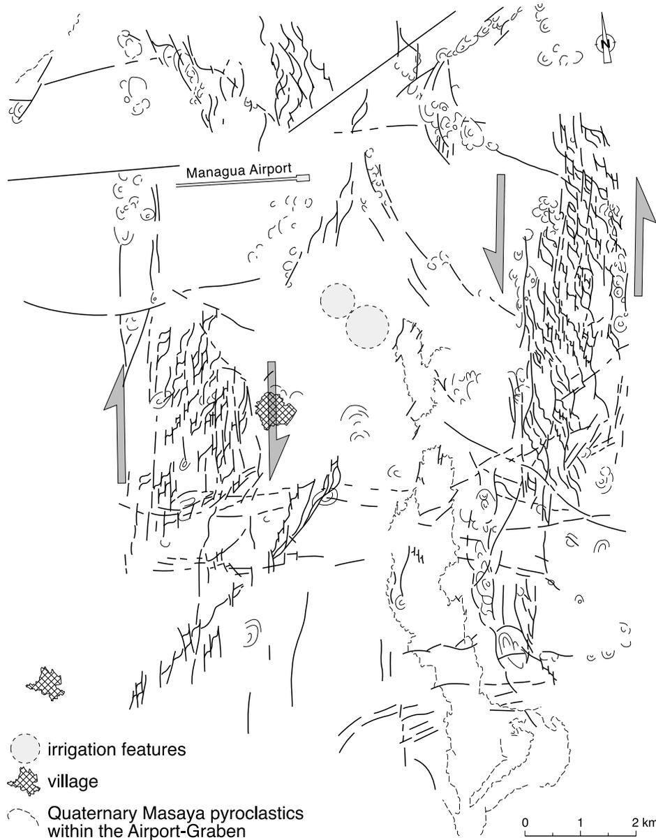
Fig. 6. Interpretation of a SPOT-image for the area of the Airport graben near Managua, which represents the eastern marginal structure of the Managua Fault Zone.
