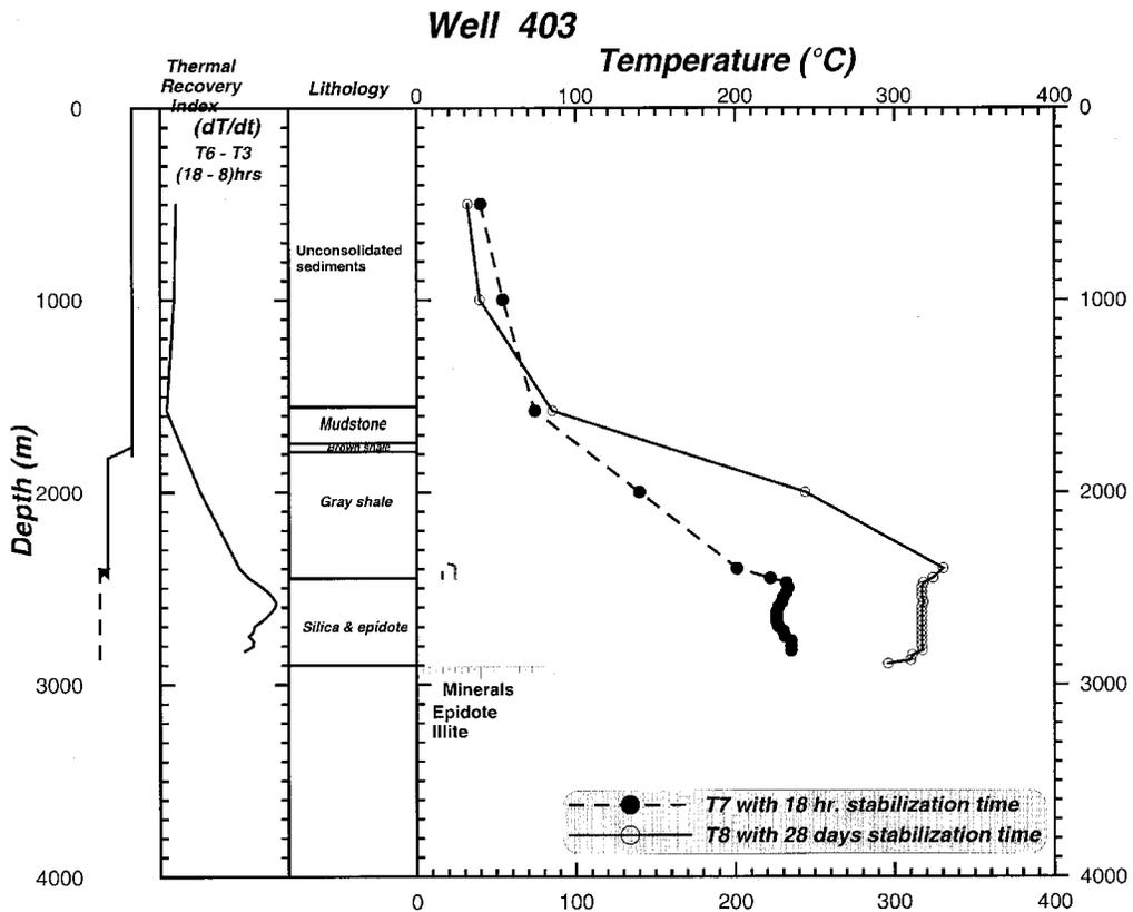
Fig. 4. Heating index profile, well completion, circulation loss profile, lithology and temperature logs for well 403.
