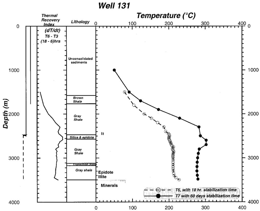
Fig. 3. Heating index profile, well completion, circulation loss profile, lithology and temperature logs for well 131.
