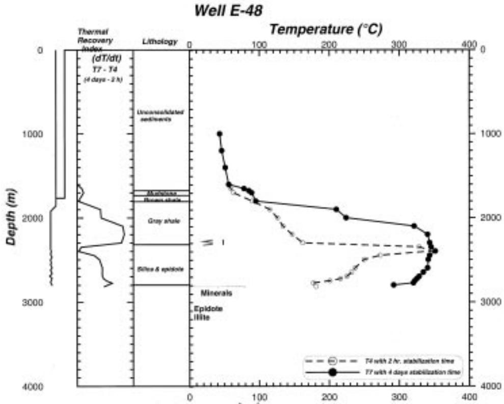
Fig. 5. Heating index profile, well completion, circulation loss profile, lithology and temperature logs for well E-48.
