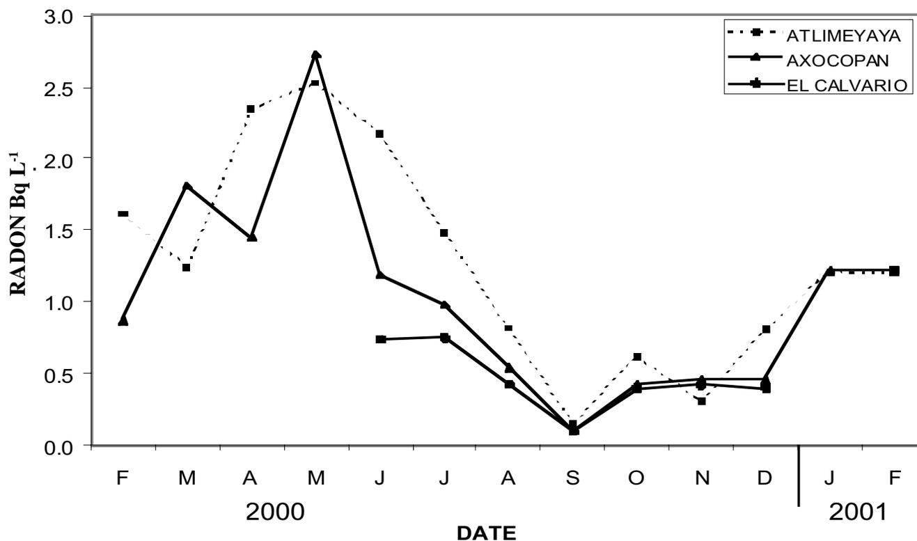
Fig. 3. Radon concentration (Bq L<sup>-1</sup>) in the water samples at Atlimeyaya, Axocopan and Calvario during 2000-2001.
