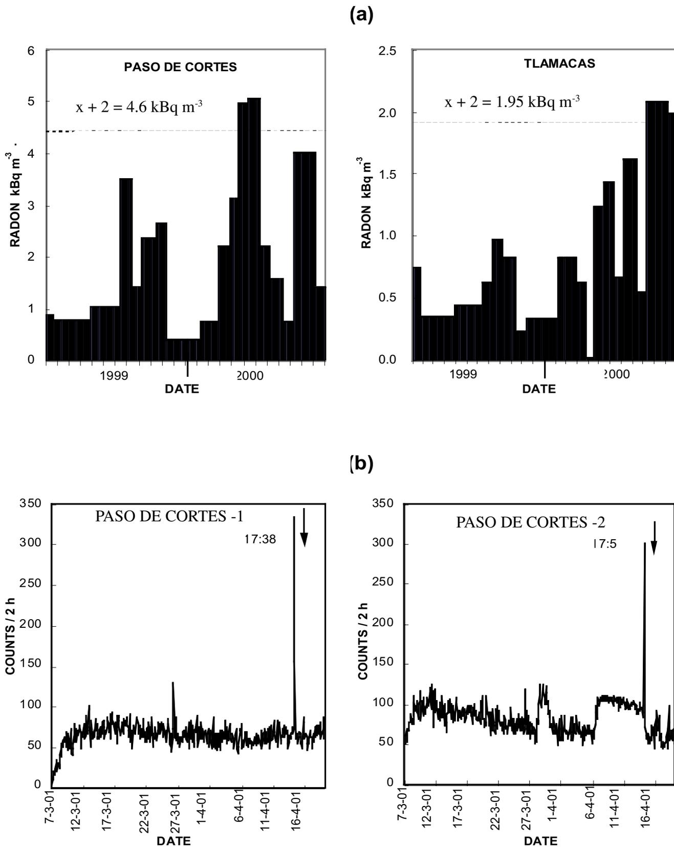
Fig. 2. (a) Soil radon at Tlamacas and Paso de Cortés during 1999-2000. (b) Radon signals from the Clipperton instrument. The peak occurred 2 days before the eruption (arrow).
