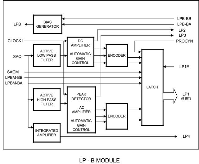
Fig. 5. Block Diagram of the LP MODULE-B.
