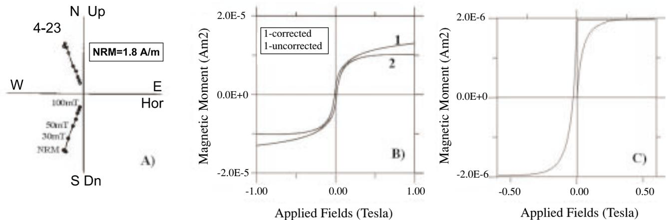
Fig. 2. A) Typical example of alternating field demagnetization vector plot for Paricutín lavas. B) Example of hysteresis curve measured with 'AGFM-Micromag' system. C) Example of direct field isothermal remanent magnetization (IRM) acquisition curve and back-field curve.
