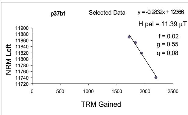
Fig. 3 and 4. Results from the microwave intensity analyses:  $f$ ,  $g$  and  $q$  are the fraction of extrapolated NRM used, the gap factor and quality factor (Coe *et al.*, 1978) respectively. Open/close symbols devote to the points rejected/used for paleointensity determination.
