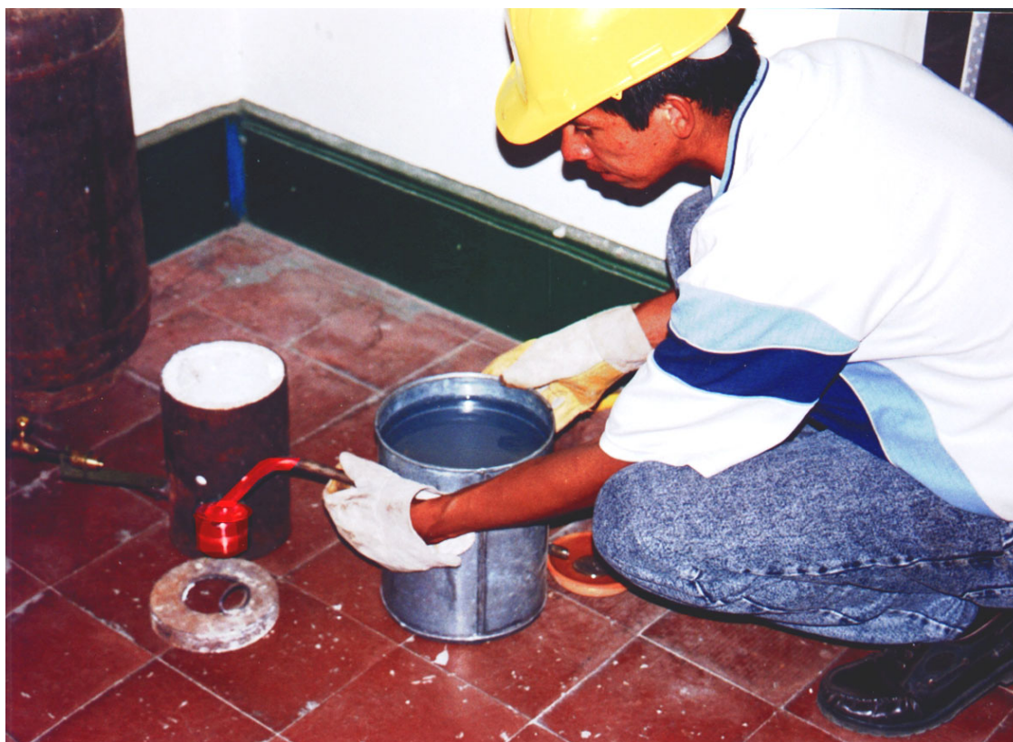
Fig. 4. Gold recovery unit (gas-fired version).
