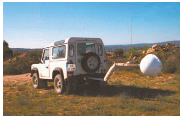
Figure 7. VLF-EM method: equipment adapted to a vehicle (Castelejo mining site).
